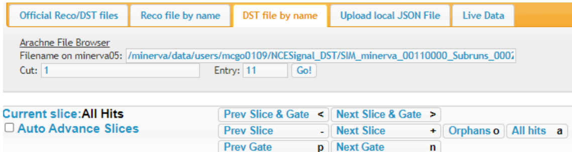
FIGURE 4.1: Any stored DST file can be viewed by inputting its path into the Filename search bar
