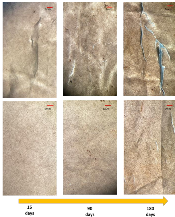
Figure 12 Films pictured at 12x magnification after 15, 90 and 180 days in aerated static-compost. Plasma treated BMF (top) shows signs of fragmentation whereas untreated films (bottom) show lower degree of degradation over this same time.
