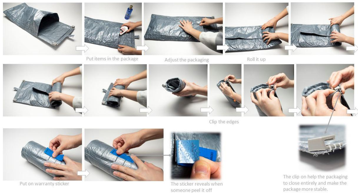
*Figure 12:Packing Processes of the Final Solution*
