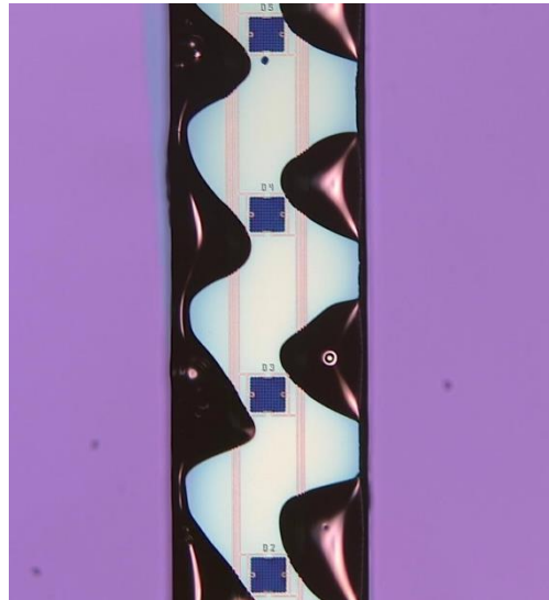
Figure 33. Sensor array with epoxy covering line-resistor contacts
