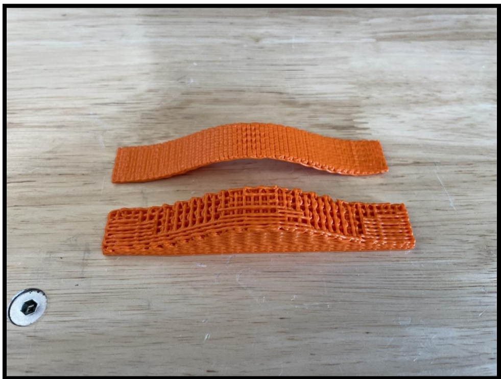
Figure 74 Removing Support from Non-Planar Part
