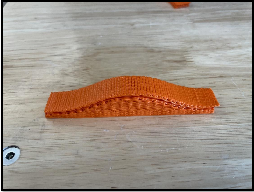
Figure 73 Non-Planar Part Printed On A Support Structure
