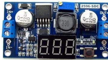
Figure 20: LM2596S DC-DC step-down buck converter
