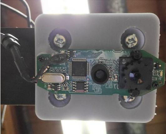
**Figure 22:** Up close view of the web camera system and mounting fixtures.
