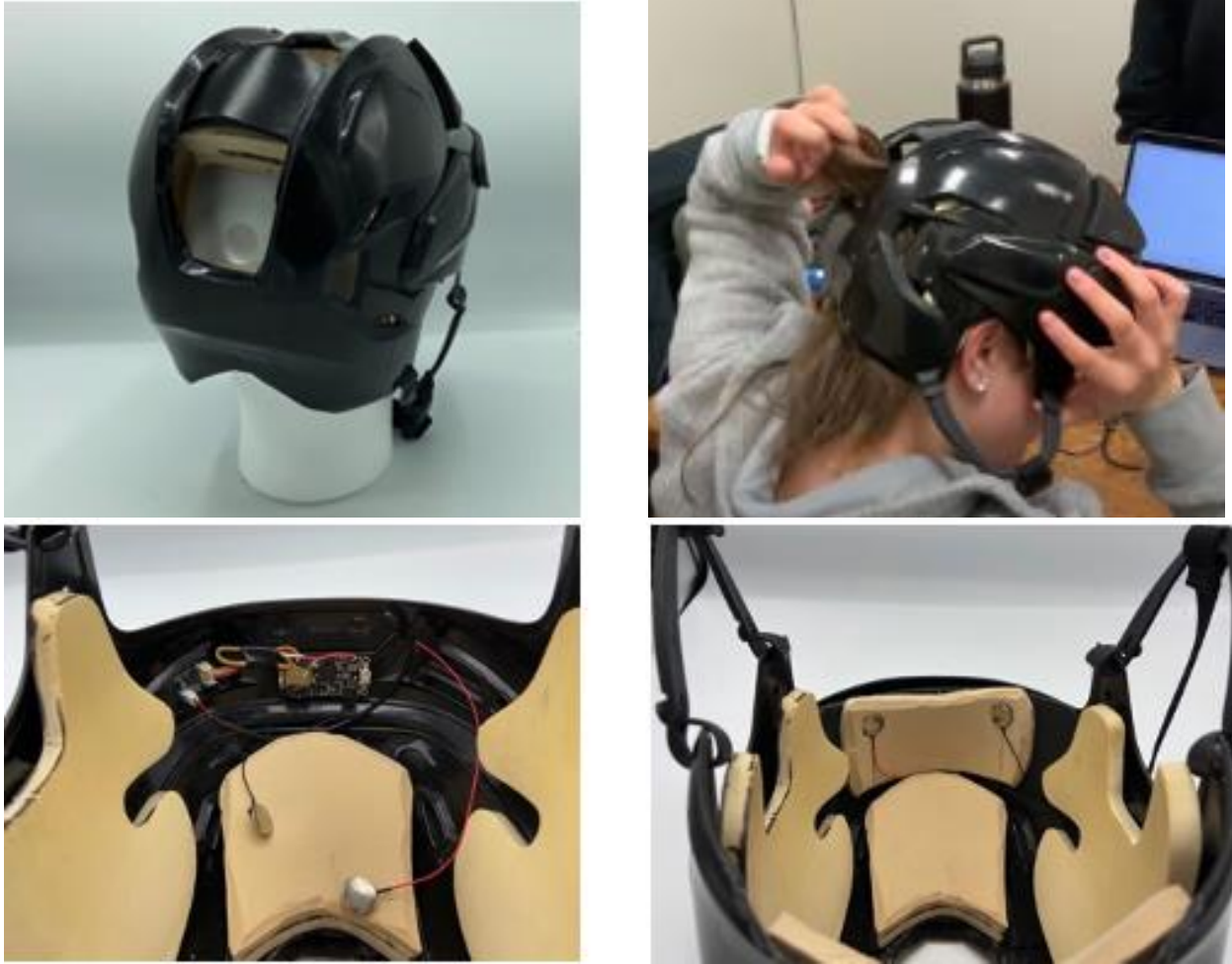
Figure 13 – Smart helmet prototype with embedded galvanic sensor
