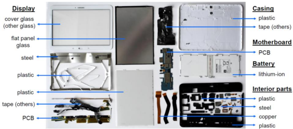
Figure 2.1 Example of product disassembly for a tablet (Samsung Galaxy Tab 4 SM-T530, 2014), illustrating the disaggregation achieved via lab disassembly and physical identification and measurement of representative assemblies (underlined terms), components, and materials.
