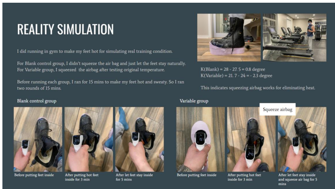
Fig. 6 Airflow efficiency test
