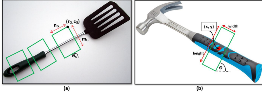
Figure 3.2: Grasping rectangle representations. (a) The representation by Jiang et al. [8]: Top vertex (r_G, c_G) , length m_G , width n_G and its angle from the x-axis, for a kitchen utensil. There can be multiple ground-truth grasps defined as shown. (b) The simplified representation by Redmon et al. [9] for a hammer, showing its grasp centre at (x, y) oriented by an angle of \theta from its horizontal axis. The rectangle has a width and height of w and h respectively.
