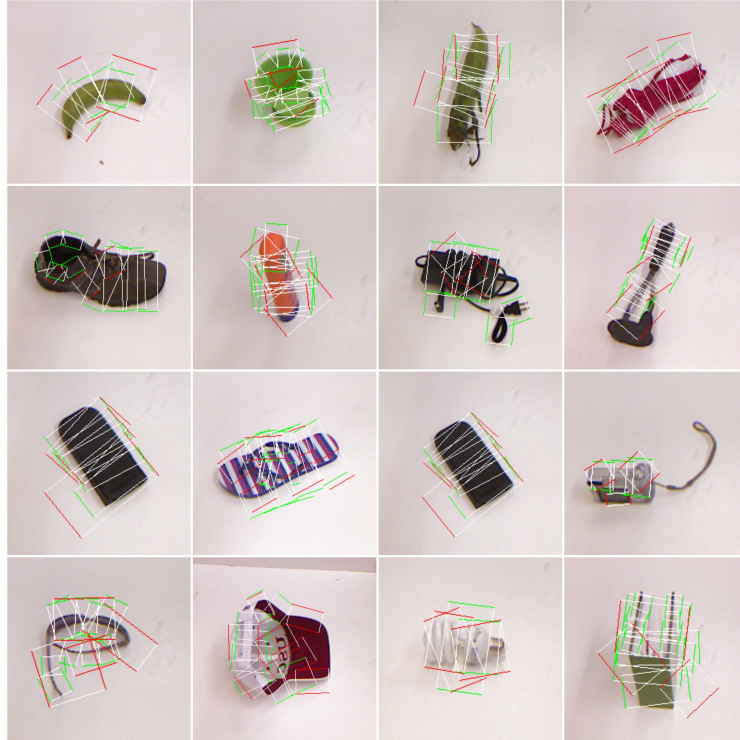
Figure 4.6: Ground truth grasps using the rectangular metric for a subset of the CGD.
