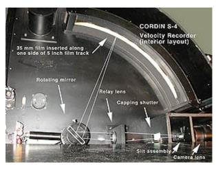
reducing the subject to a single line, e.g. limiting the height or width of the subject either inside the camera with a slit or at the subject with physical masks. The displacement in time is obtained by reflecting the image of that line off a mirror that can be made to rotate at a rapid rate onto film that is installed in an arc around the center of rotation of the mirror.
