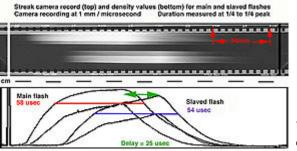
1/333.3 seconds. The rate of image motion on the film is, therefore, 3265 mm / 1/333.3 sec. which is 1,088,224 mm/sec or, to simplify matters, 1 mm in 1/1,000,000 second.
