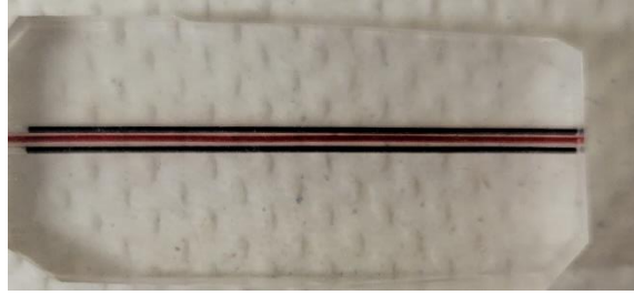
Figure 35. Planar microchip fabricated using three microfibers. Approximate spacing is between 400 – 500 \mu\text{m} . Food coloring is used to show discrete channels.
