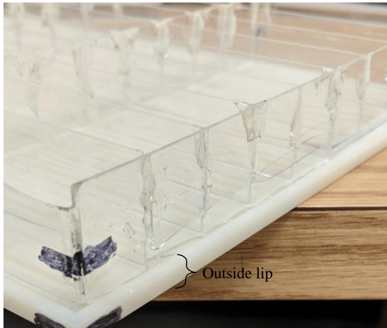
Figure 13. Damaged glass slides of outside walls. The lip designed to lock the glass slides in place caused the damage.
