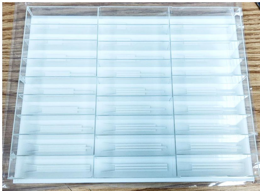
Figure 12. Mold array with installed and glued standard microscope slides (25 mm by 75 mm by 1 mm).
