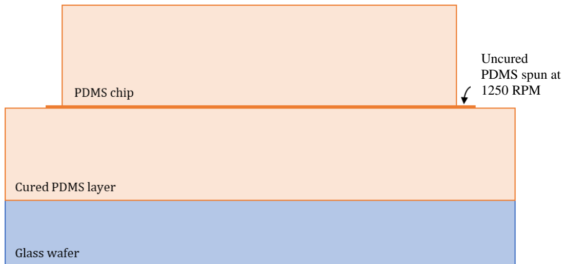
Figure 20. Schematic of a small section depicting PDMS-PDMS bonding.
