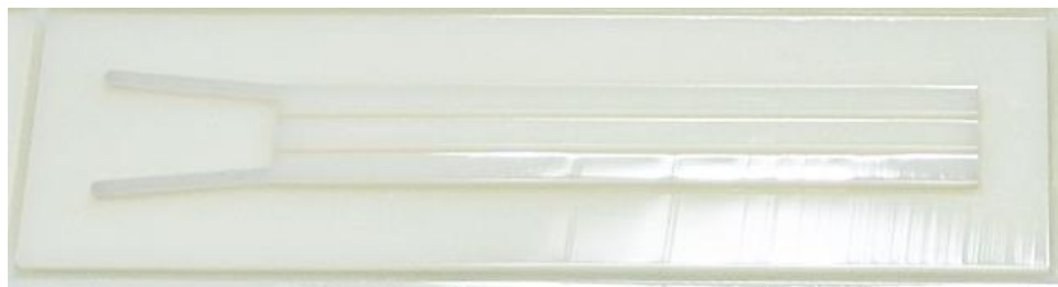
Figure 11. Gloss finish of SLA 3D printed negative mold.
