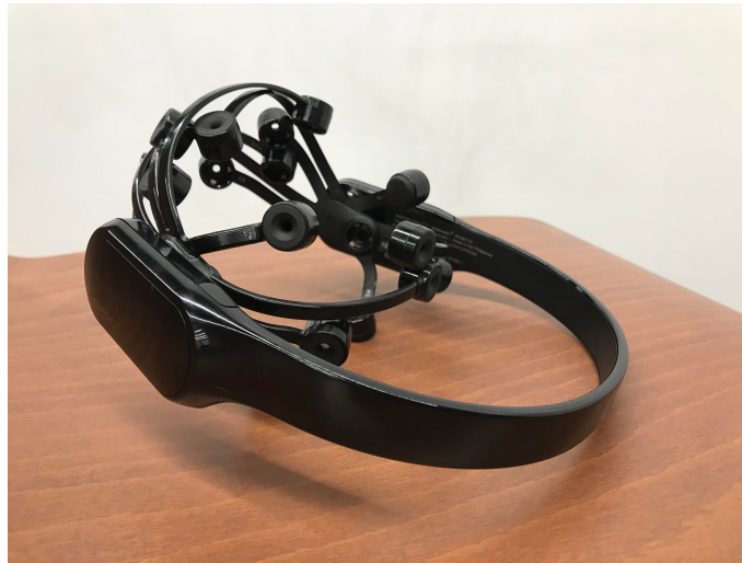
Figure 4.1: EEG cap (EPOC X) with 14 channels. The sensor felts are hydrated with a saline solution, and then are inserted into each channel for improving the conductivity, reducing the skin-electrode impedance.
