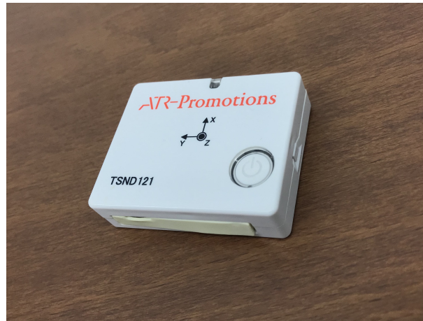
Figure 3.1: The small wireless multi-functional sensor (TSND121), which can measure the acceleration data and transmit it through a Bluetooth wireless link.
