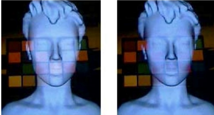
Figure 2.4: Image captured by a webcam through the OST display rendering a bust with color checker on the background by Weiland et al. [27] Left is the uncompensated rendering with color distortion. The right is compensated rendering with background subtraction.
