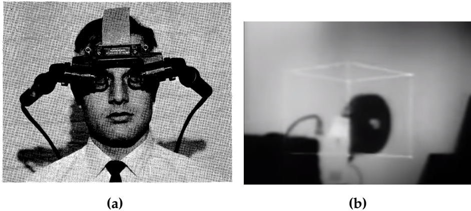
Figure 2.1: (a) The AR head-mounted 3D display in 1968 by Sutherland and his team.[5] (b) A virtual cube with real world background through the display. Image from ACM Fall Joint Computing Conference, San Francisco 1968.
