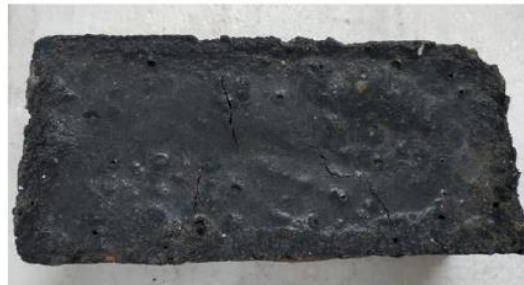
Figure 5: Samples of plastic concrete blocks (Hassanien, 2020).
