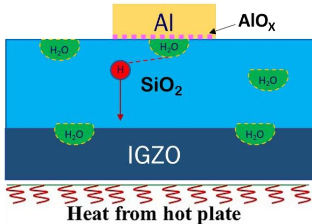
Figure 3.9: Proposed mechanism of thermal degradation. Monatomic hydrogen is generated by a reaction between  $H_2O$  and the top-gate metal in DG TFTs, and diffuses to the back-channel region [13].  $AlO_x$  forming at the interface of the Al top gate and the passivation oxide.
