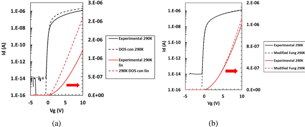
Figure 4.5: (a) DOS continuity with  $W_{TA}=13\text{meV}$  at RT (b) without DOS continuity using  $W_{TA}=13\text{meV}$  at RT (reproduction of Figure 2.10).
