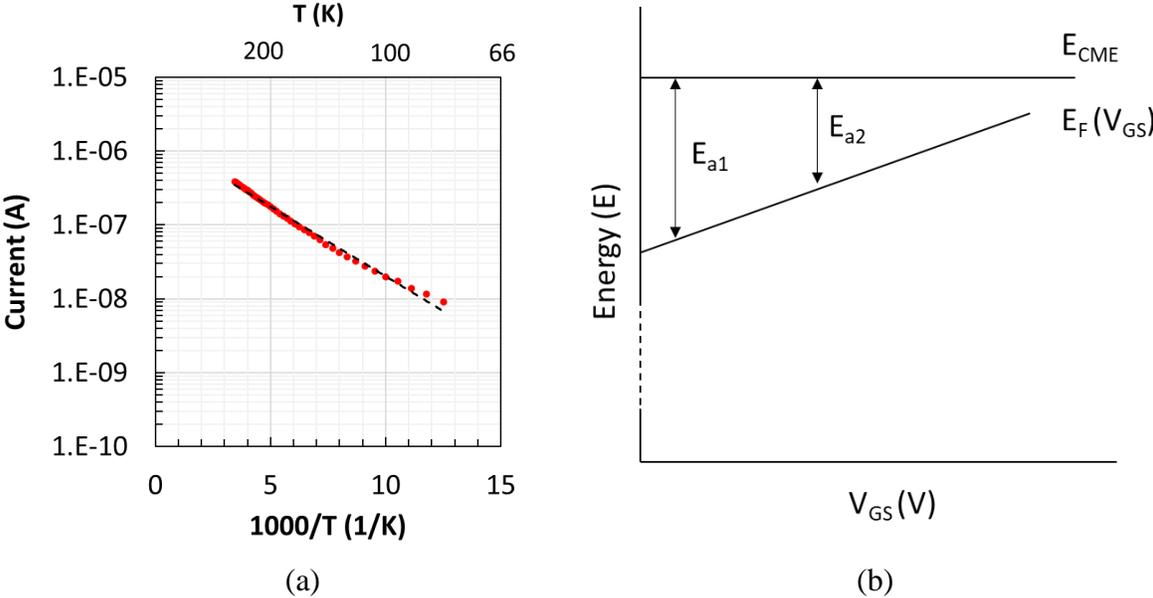
Figure 4.2: (a) Drain current versus temperature plot at  $V_{DS}=0.1$  V and  $V_{GS}=5$  V. Charge transport follows Arrhenius behavior for  $T > 100$  K, indicating thermally activated band conduction as the charge transport mechanism. (b) Conceptual representation of energy versus gate voltage. Increasing gate voltage causes  $E_F$  to approach the conduction band mobility edge.
