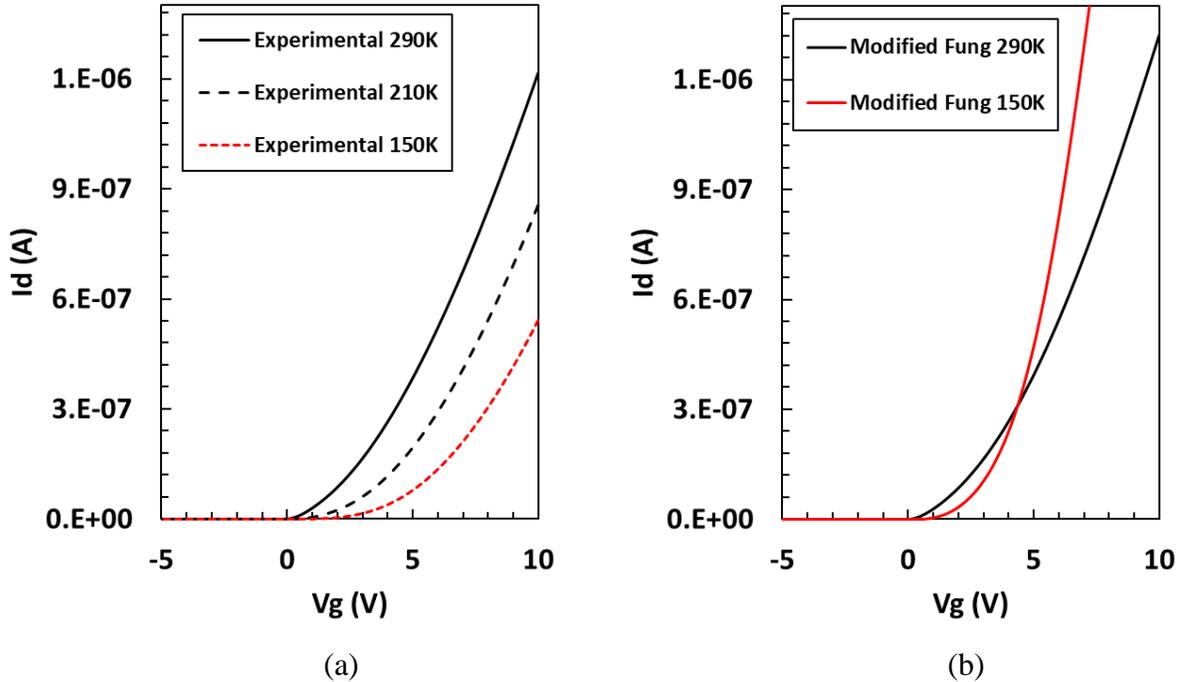
Figure 4.6: (a) Experimental transfer characteristics at different temperatures, (b) Simulated I-V characteristics using modified passivated parameters and default (Fung) mobility model.
