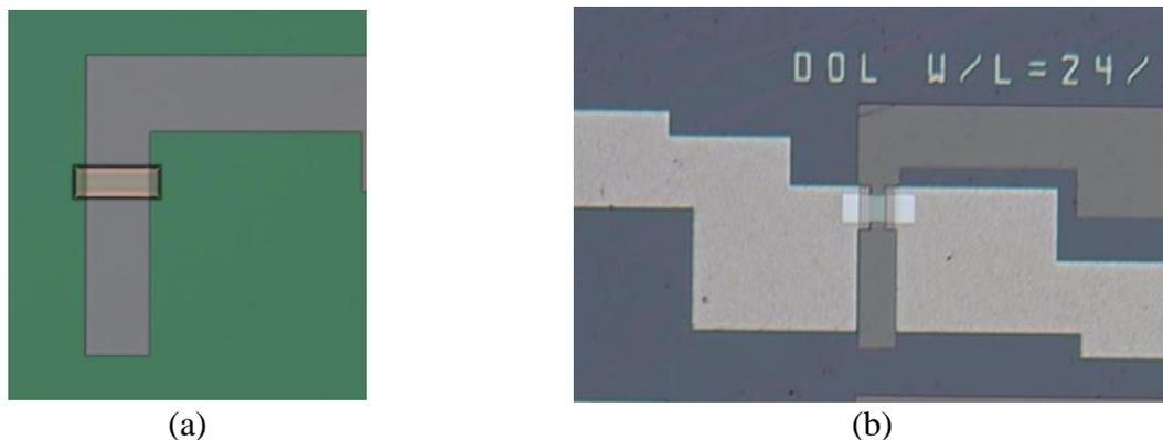
Figure 7.16: (a) Wet etched ITGO active region (wet etch rate 20nm/min), (b) Completed BG ITGO TFT showing transparent channel region.
