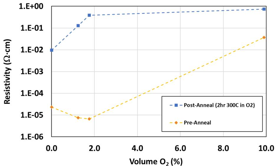
Figure 7.7: Resistivity vs. %O<sub>2</sub>, annealed in dry O<sub>2</sub> at 300°C for 2 hr. Note R<sub>s</sub> measurements converted to the material resistivity (Ω·cm).
