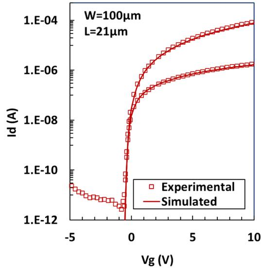
Figure 2.8: Unpassivated TFT showing excellent match with TCAD simulated characteristics using modified unpassivated TCAD parameters from Table 2-III [25].
