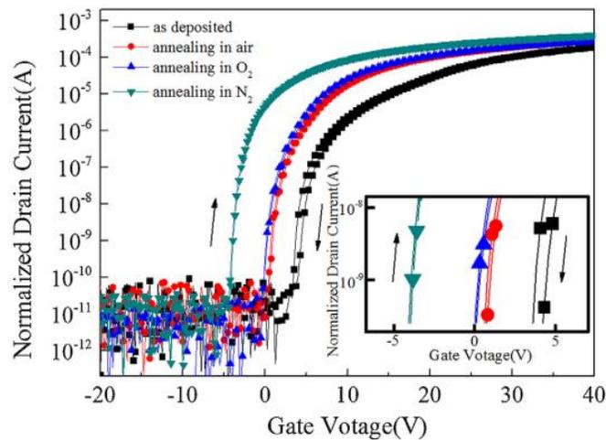
Figure 7.5: Transfer characteristic curves of a-IWO TFTs under different annealing ambient conditions [122]
