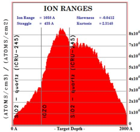
Figure 6.11: Representative SRIM analysis of <sup>11</sup>B<sup>+</sup> implanted with energy  $E = 35$  keV into IGZO beneath a 50 nm screen SiO<sub>2</sub> layer. The simulation shows that approximately 40 percent of the implanted dose resides within the IGZO film, which translates to an average boron concentration of approximately  $3.2 \times 10^{20}$  cm<sup>-3</sup> [99].
