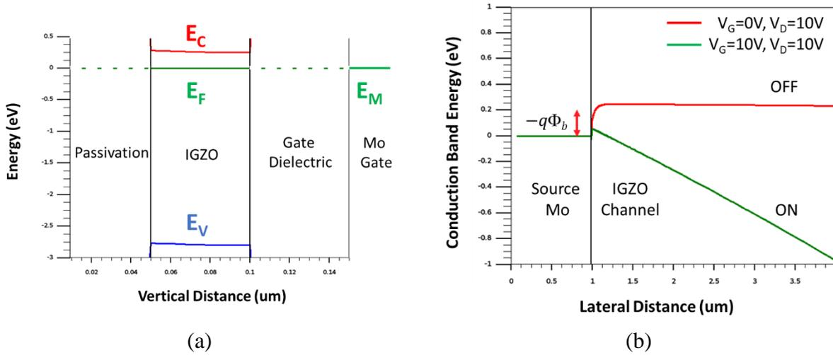
Figure 2.7: (a) Energy band along the thickness of the device showing conduction band ( $E_C$ ), valence band ( $E_V$ ), Fermi level ( $E_F$ ), metal level ( $E_M$ ) where  $V_{DS}=V_{GS}=0V$ , the electron concentration is  $\sim 10^{14} \text{ cm}^{-3}$  and (b) Conduction band energy near the source end of the device showing for  $V_G=0$  &  $10V$  at high drain bias ( $V_{DS}=10V$ ).
