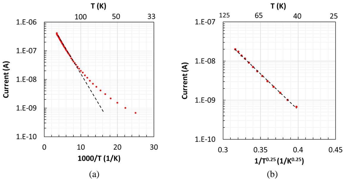
Figure 4.1: (a) Drain current versus  $1000/T$  shown for the full temperature (40K-290K) regime, it can be seen that at lower temperatures the current no longer follows a linear relationship with reciprocal temperature & (b) The linear dependence of  $\log(ID)$  on  $1/T^{0.25}$  over temperature (40K- 100K) indicates variable range hopping as the carrier transport mechanism at low temperature ( $T < 100$ K). Here,  $V_{DS} = 0.1$  V and  $V_{GS} = 5$  V.
