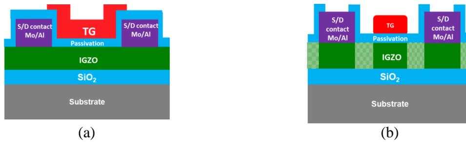
Figure 6.1: Cross sectional image of (a) non-SA TG TFT and (b) SA-TG TFT (The patterned region indicates the ion-implanted mesa).
