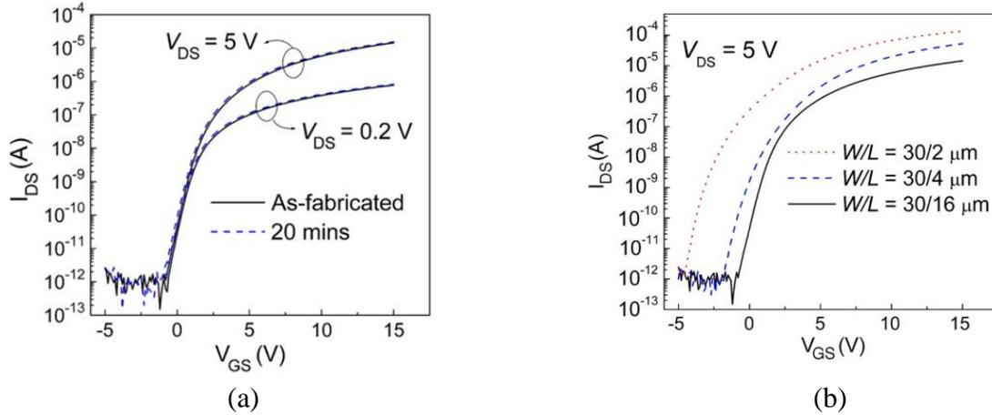
Figure 6.8: (a) Transfer characteristics of the IGZO TFTs with arsenic doped S/D regions under thermal stress treatment for 20 min at 200 °C ( $W/L=30/16$ ) and (b) transfer characteristics of the IGZO TFTs with the same channel width but different channel lengths. Adapted from [98].
