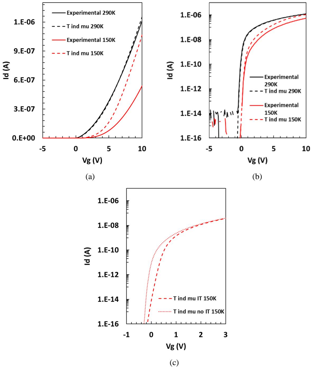
Figure 4.7: Temp independent mobility 290k vs 150k, where the mobility  $\mu=19\text{cm}^2/\text{Vs}$  in (a)linear scale, (b)log scale &(c) Simulated I-V with or without IT at  $T=150\text{K}$ .
