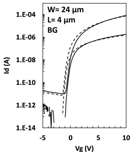
Figure 5.3: Transfer characteristics of an intermediate stage (gate oxide thickness remained at  $100\ \text{nm}$  and the passivation oxide thickness was reduced to  $50\ \text{nm}$ ) BG device shown here in dashed line compared with device with gate oxide thickness and the passivation oxide thickness at  $100\ \text{nm}$  where each has  $W = 24\ \mu\text{m}$  and  $L = 4\ \mu\text{m}$  [58].
