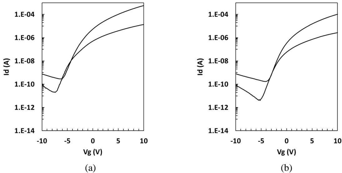
Figure 7.17: ITGO TFT characteristics a)  $L=12\mu\text{m}$  and b)  $L=48\mu\text{m}$  with  $t=50\text{nm}$  &  $P_{O_2} = 10\%$  and annealed at 300C for 2hr in O<sub>2</sub>
