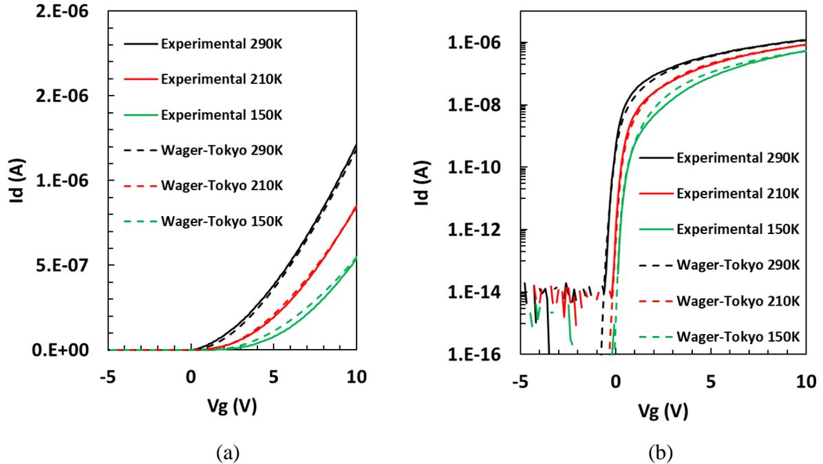
Figure 4.14: Hybrid BTS-IGZO.Tokyo model results with adjusted parameters (Table 4-II, column 3)
