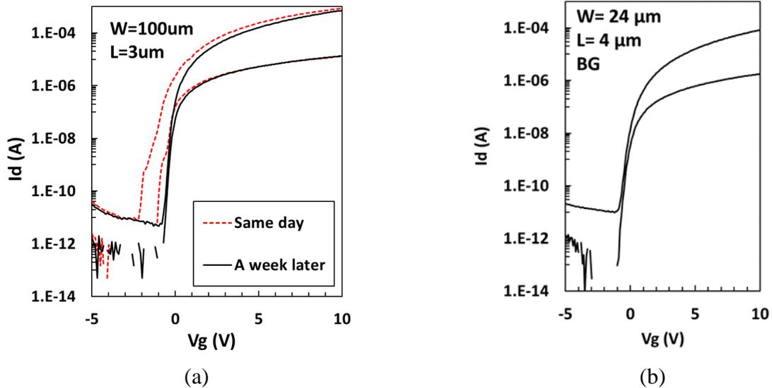
Figure 2.2: Transfer characteristics of IGZO TFTs with BG configuration (a) Unpassivated [25] & (b) Passivated device [26]. Drain bias conditions are 0.1V and 10V.
