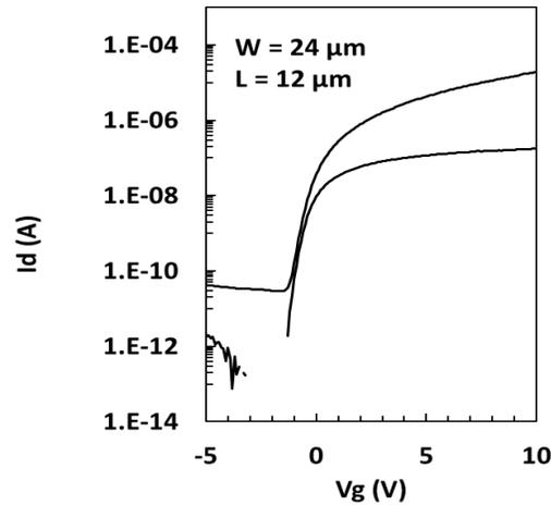
Figure 6.18:  $^{11}\text{B}^+$  implanted ( $\phi = 4 \times 10^{15} \text{ cm}^{-2}$ ) pseudo-SA BG device characteristics with  $L = 12 \mu\text{m}$ . The device width is  $24 \mu\text{m}$  and the  $V_d$  is 0.1 and 10 V respectively with  $4 \mu\text{m}$  underlap between BG and S/D contact metal.
