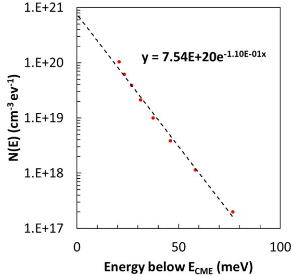
Figure 4.3: Extracted DOS ( $N(E)$ ) versus energy below the conduction band mobility edge.
