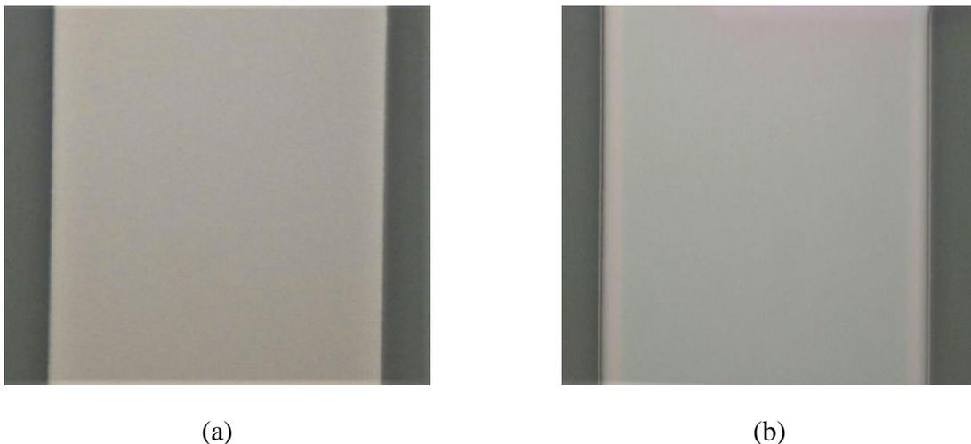
*Figure 6.20: BG pattern (a) without backside flood exposure and (b) with backside flood exposure. Note that, resist is remaining everywhere without the backside flood exposure whereas resist is only remaining on top of BG polygon with the backside flood exposure.*
