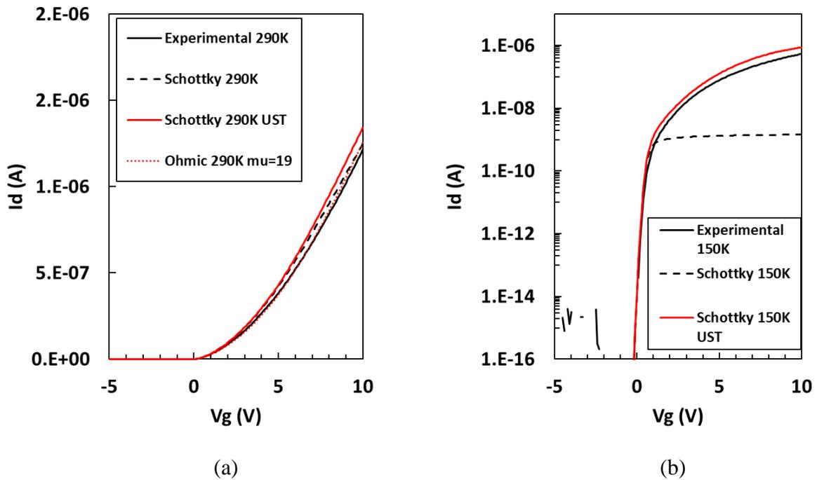
Figure 4.9: Measured and simulated transfer characteristics at (a)  $T = 290$  K and (b)  $T = 150$  K, with  $V_{DS} = 0.1$  V and indicated parameter treatment combinations for Schottky barrier ( $q\Phi_M = 4.35$  eV), Ohmic ( $q\Phi_M = 4.13$  eV), with and without UST, and intrinsic channel mobility ( $\mu_{ch}$ ) adjusted to  $23\text{cm}^2/\text{Vs}$  unless indicated otherwise.
