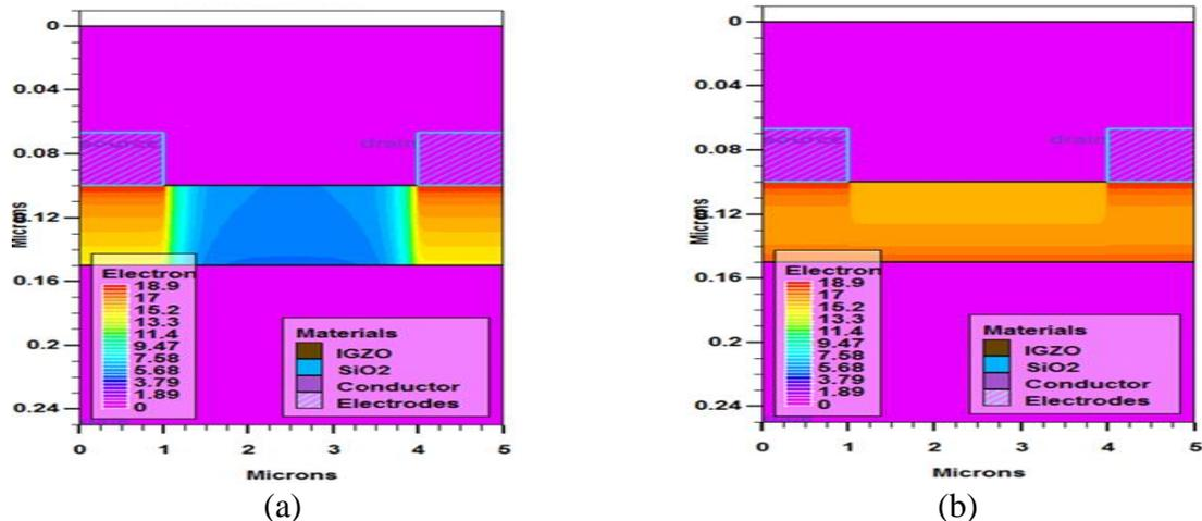
Figure 3.17: ATLAS simulation showing electron concentration of BG TFTs in (a) un-biased state and in (b) positive-stress [60].
