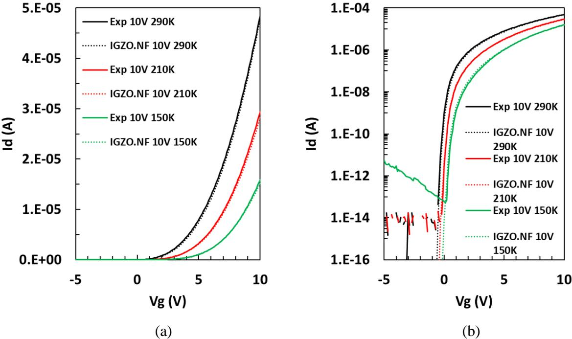
Figure 4.17: Non-Fermi mobility model with mobility as a function of temperature with  $V_D=10V$ .
