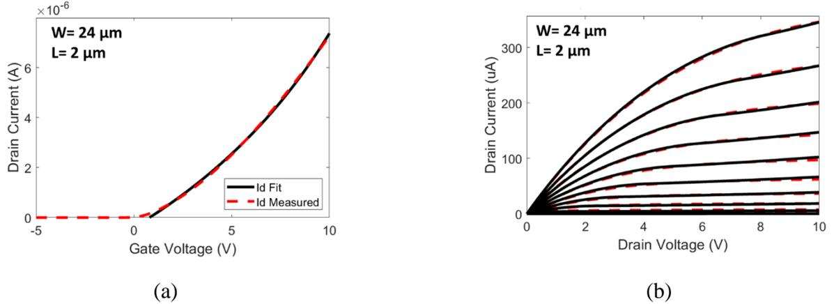
Figure 5.6: BTS2D device model representing the on-state operation of a BG device with 2  $\mu\text{m}$  channel length, showing an excellent fit to the linear-mode transfer characteristic (low drain bias) and output characteristic family of curves [58].
