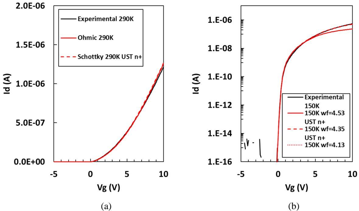
Figure 4.21: (a) Schottky contact with UST & n+ interface and Ohmic contact show perfect match with experimental results at room temperature, here  $\mu_0=19 \text{ cm}^2/\text{Vs}$ , (b) At 150 K,  $wf=4.13 \text{ eV}$  shows an almost perfect overlay with experimental results and simulated I-V using higher workfunctions with UST & n+ interface here  $\mu_0=9 \text{ cm}^2/\text{Vs}$ .
