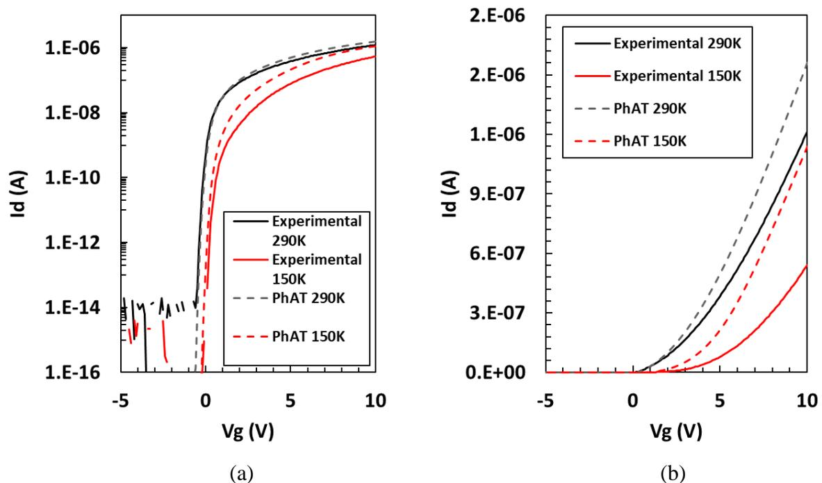
Figure 4.11: PhAT model 290K & 150K simulated vs experimental data.
