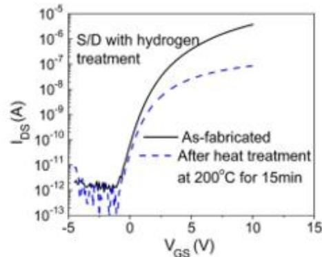
Figure 6.4: Transfer characteristics of the IGZO TFTs with S/D regions treated with hydrogen plasma under heat treatment at  $200 \text{ }^\circ\text{C}$ . Adapted from [95].
