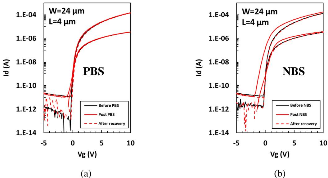
Figure 5.8: Two separate BG devices showing effects of (a) PBS and (b) NBS applied at  $V_G = \pm 10$  V with S/D at reference ground. The post-stress measurements were taken immediately following 1 hour stress duration. The PBS effect is virtually negligible, whereas the NBS effect indicates the influence of carrier traps. Both PBS and NBS effects were completely reversible [58].
