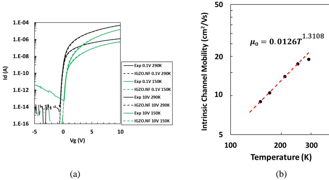
Figure 8.1: (a) Low drain & high drain for 290K and 150K using IGZO.NF model with mobility as a function of temperature and (b) Power law fit of mobility extracted from IGZO.NF model as a function of temperature, at room temperature  $\mu_0=19\text{cm}^2/\text{Vs}$  and at 150K  $\mu_0=9\text{cm}^2/\text{Vs}$ .
