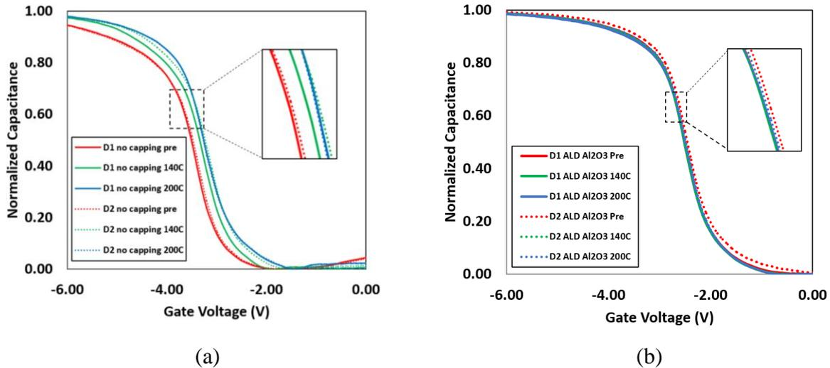
Figure 3.10: C-V characteristics of MOSCAPs (a) without capping layer and (b) with  $Al_2O_3$  capping layer. Without capping, they show  $\sim 0.4$  V shift in  $V_{FB}$  and with  $Al_2O_3$  capping, the  $V_{FB}$  shift is  $\sim 0$  V. Note that C-V characteristics from two separate devices are shown for each treatment [13].
