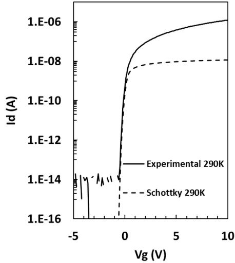
Figure 4.8: Workfunction=4.53 used for S/D contact shows Schottky contact and the simulated I-V shows contact limited behavior at room temperature.
