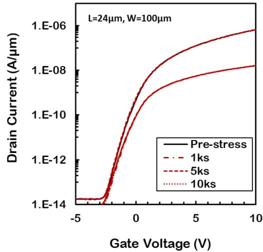
Figure 3.16: BG device under the influence of PBS showing no effect on device characteristics [40].
