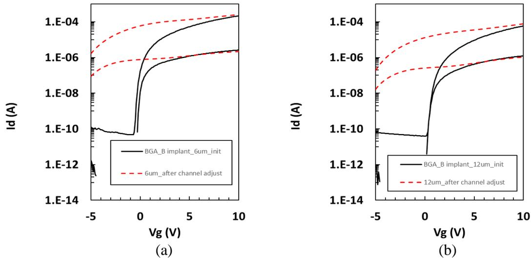
Figure 6.24: Comparison of low dose ( $\phi = 2 \times 10^{12} \text{ cm}^{-2}$ )  $^{11}\text{B}^+$  implant on  $\phi = 4 \times 10^{15} \text{ cm}^{-2}$   $^{11}\text{B}^+$  implanted SA-BG device characteristics for  $V_T$  adjust with (a)  $L = 6 \mu\text{m}$  and (b)  $L = 12 \mu\text{m}$ . The device width is  $24 \mu\text{m}$  and the  $V_d$  is 0.1 and 10 V respectively with  $4 \mu\text{m}$  underlap between BG and S/D contact metal.
