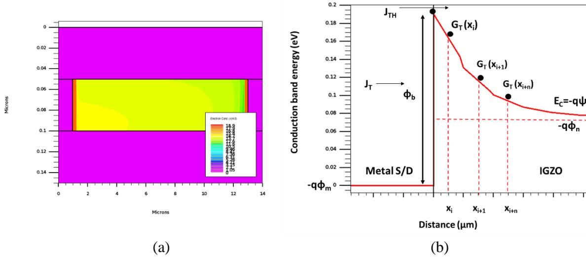
Figure 4.10: (a) BG TFT with edge-defined contact regions for barrier simulation, here  $V_D=1V$  and  $V_G=0V$ , (b) Conduction band energy showing tunneling and thermionic emission, here  $V_D=1V$ ,  $V_G=3V$  and  $q\Phi_M = 4.35 eV$ .
