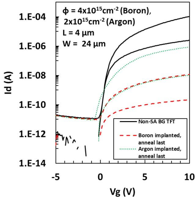
Figure 6.26: Characteristic overlay of an anneal-last SA-BG device with boron and argon doping and a non-SA-BG TFT with the same channel dimensions as indicated [106].
