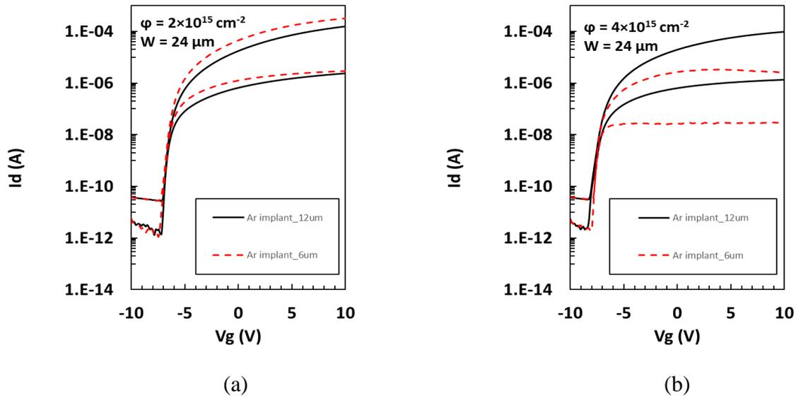
Figure 6.13: Comparison of  $^{40}\text{Ar}^+$  implanted SA-TG device characteristics with  $L = 6$  (red dashed line) and  $L = 12 \mu\text{m}$  (black solid line) with (a)  $\phi = 2 \times 10^{15} \text{ cm}^{-2}$  and (b)  $\phi = 4 \times 10^{15} \text{ cm}^{-2}$  and energy  $E = 80 \text{ keV}$ . Here, the device width is  $24 \mu\text{m}$  and the  $V_d$  is  $0.1$  and  $10 \text{ V}$  respectively with  $4 \mu\text{m}$  underlap between TG and S/D contact metal.
