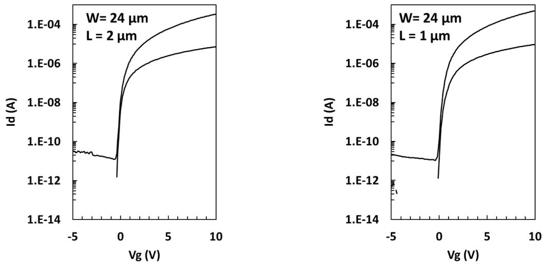
Figure 5.4: Transfer characteristics from BG devices fabricated with the revised process which included gate oxide thickness reduction to 50 nm. Excellent performance is demonstrated at  $2 \mu\text{m}$  and  $1 \mu\text{m}$  channel lengths, as suggested by Table 5-1 [26].
