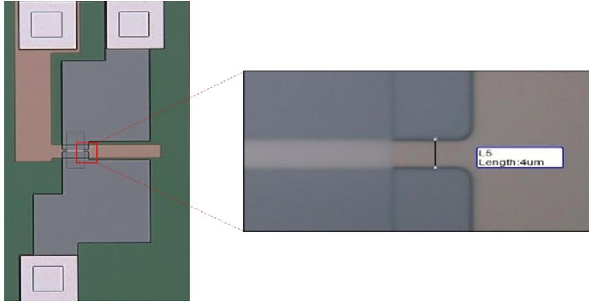
Figure 5.1: BG IGZO TFT with channel length  $L = 4 \mu\text{m}$  as defined by the S/D lift-off metallurgy using negative photoresist (Futurrex NR9g-1500PY) with almost negligible offset from the mask definition (i.e.  $\Delta L \sim 0$ ) [58].
