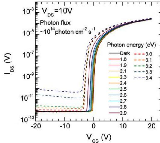
Figure 3.1 Transfer characteristics of IGZO TFTs in dark and under monochromatic light illumination with photon energies ranging from 1.8 eV to 3.4 eV ( $\lambda=700\text{-}365\text{ nm}$ ). Adapted from [45].
