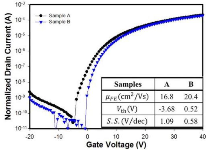
Figure 7.3: Transfer curves of a-IWO TFTs: samples A and B, at  $V_{DS}=10\text{V}$ . The Inset shows the electrical parameters, including carrier mobility, threshold voltage and subthreshold swing [120].
