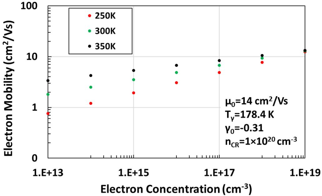
Figure 4.12: Mobility vs concentration at varied temperature using equation 4.19 and 4.20.
