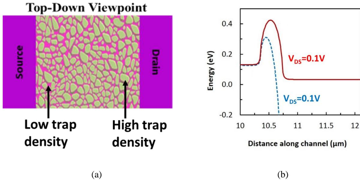
Figure 3.5: (a) Schematic model for the TABL origin, showing a cobblestone arrangement of donor-rich interface defect regions separated by low-charge gaps [40]. (b) Conduction band energy across the channel at low and high drain bias showing the barrier created by the low charge pocket (gap). At high drain bias (dashed line) the barrier is lowered [25].
