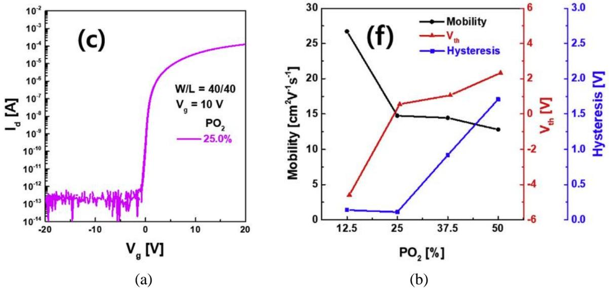
Figure 7.12: (a) Transfer curves of ITGO TFTs with  $P_{O_2} = 25\%$  and (b) field-effect mobility, threshold voltage, and hysteresis of the ITGO TFTs as a function of  $P_{O_2}$ , adapted from [133].
