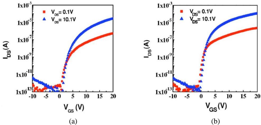
Figure 6.5: Representative transfer characteristics ( $W/L=50/4 \mu\text{m}$ ) of IGZO TFTs (a) without and (b) with Ar plasma treatment before depositing the source/drain electrode. Adapted from [90].
