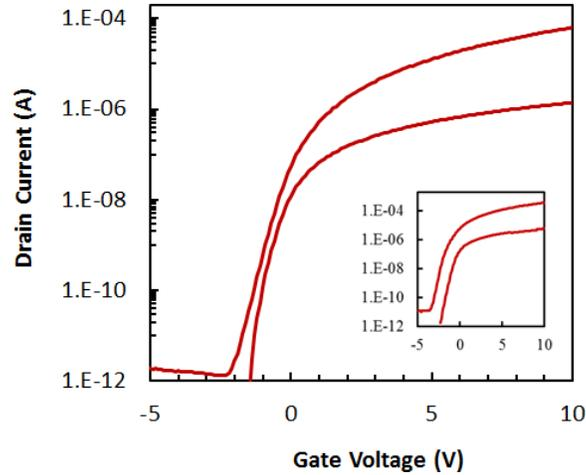
Figure 3.3: Measured data for a  $L=21\ \mu\text{m}$  BG device with  $100\ \text{nm}$   $\text{SiO}_2$  passivation, showing TABL. Inset shows the transfer characteristics for  $L=3\ \mu\text{m}$  device showing pronounced distortions for a scaled device [40].
