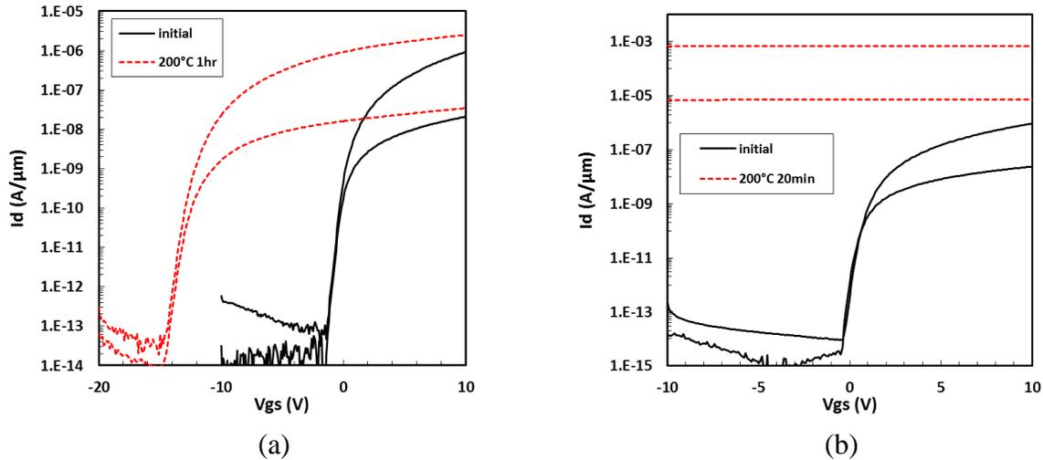
Figure 3.8: (a) BG and (b) DGL  $L = 24 \mu\text{m}$  devices with  $\text{SiO}_2$  back-channel passivation that demonstrate performance degradation or failure after 200 °C thermal treatment [13].
