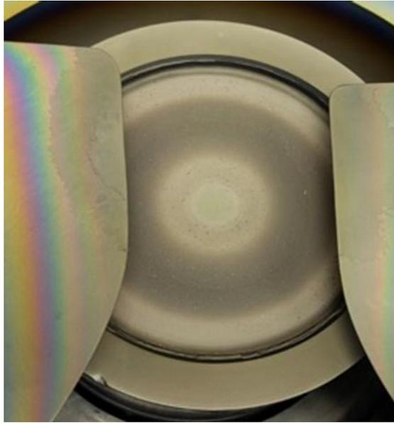
*Figure 7.4: IWO target installed in CVC601 sputter machine with added shields for improved sputter uniformity.*
