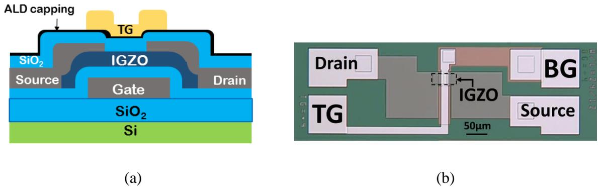
Figure 3.11: (a) Cross-section schematic of a DG TFT with ALD capping layer. The DG device has the staggered electrode configuration of the BG device, with the addition of a co-planar top gate. Note that the bottom and top gate electrodes in the DG device are electrically connected through a contact not shown. (b) Top-down view of a fabricated DG TFT. Note that the IGZO channel is highlighted [13].
