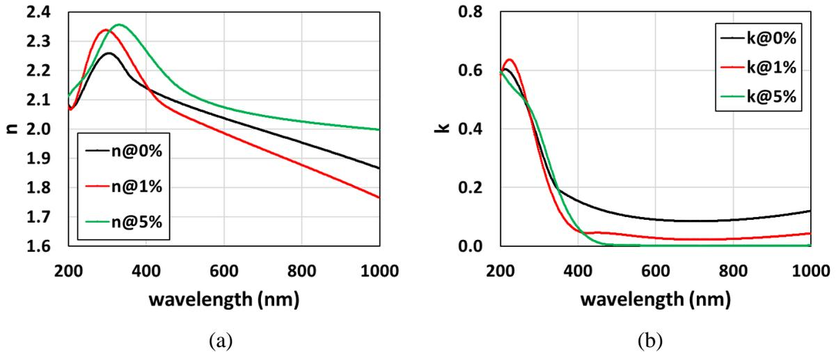
Figure 7.14: Optical constants (a)  $n$  & (b)  $k$  with varying oxygen partial pressure during ITGO sputter.
