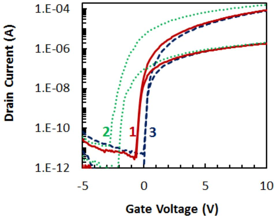
Figure 3.4: Ripened transfer characteristics (#1) as shown in Figure 3.2 followed by a partial etch of the IGZO back-channel surface, showing restoration of TABL behavior (#2). Characteristics measured after two days of ripening result in elimination of separation and distortion (#3). The shift between the initial and final ripened characteristics (#1 & #3) is attributed to the respective IGZO channel thickness[25].
