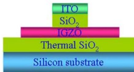
Figure 6.6: Cross-sectional schematic of the proposed IGZO TFT with SA-TG structure. Adapted from [96].
