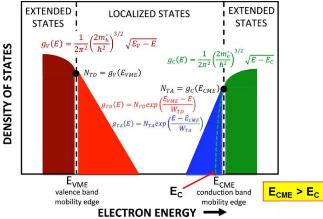
Figure 4.4: Density of states model illustrating localized and extended state densities for both valence and conduction band [70]. Here the original figure is modified to show  $E_C$  below  $E_{CME}$ .
