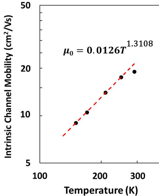
Figure 4.16: Power law fit of mobility extracted from IGZO.NF model as a function of temperature, at room temperature  $\mu_0=19\text{cm}^2/\text{Vs}$  and at 150K  $\mu_0=9\text{cm}^2/\text{Vs}$ .
