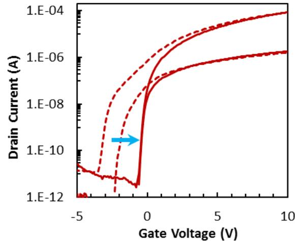
Figure 3.2: Transfer characteristics of an unpassivated TFT tested immediately after annealing (dashed line) showing TABL. After a two-day storage in room ambient the characteristics do not exhibit TABL (solid line)[40].
