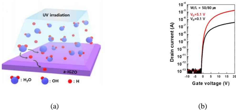
Figure 6.3: (a) Scheme of photochemical dissociation caused by DUV irradiation and (b) transfer characteristics of self-aligned coplanar IGZO TFT with DUV irradiation energy of  $30 \text{ J/cm}^2$ . The channel width ( $W$ ) and length ( $L$ ) were  $50$  and  $80 \mu\text{m}$ , respectively. Adapted from [92].
