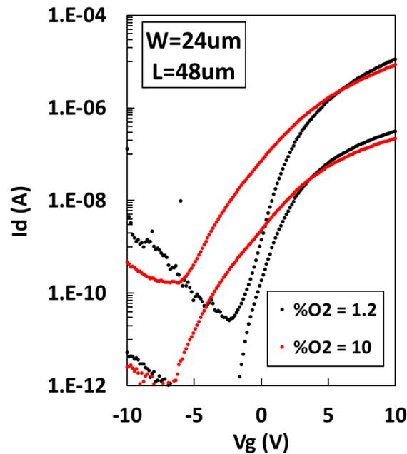
Figure 7.8: Transfer curves for 48um device sputtered in ambient of 1.2% and 10%  $O_2$  per volume and annealed dry  $O_2$  for 10-hour at 300°C.
