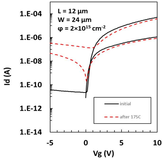
Figure 6.25: Comparison of  $^{40}\text{Ar}^+$  implanted SA-BG device characteristics with  $L = 12 \mu\text{m}$ ,  $E = 80 \text{keV}$  and  $\phi = 2 \times 10^{15} \text{cm}^{-2}$  before (solid line) and after (dashed line)  $175^\circ\text{C}$  bake for an hour [106].
