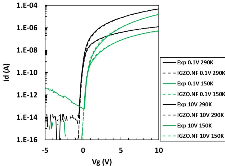
Figure 4.18: Low drain & high drain for 290K and 150K using IGZO.NF model with mobility as a function of temperature.
