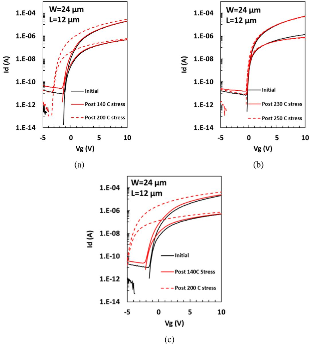
Figure 3.12: BG devices with ALD  $\text{Al}_2\text{O}_3$  capping layer deposited at (a)  $150^\circ\text{C}$ , (b)  $200^\circ\text{C}$  & (c)  $250^\circ\text{C}$ , with channel lengths and 1 hour sequential thermal stress treatment temperatures as indicated. The  $200^\circ\text{C}$  ALD temperature maintains good thermal stability at temperature up to  $250^\circ\text{C}$  [58].
