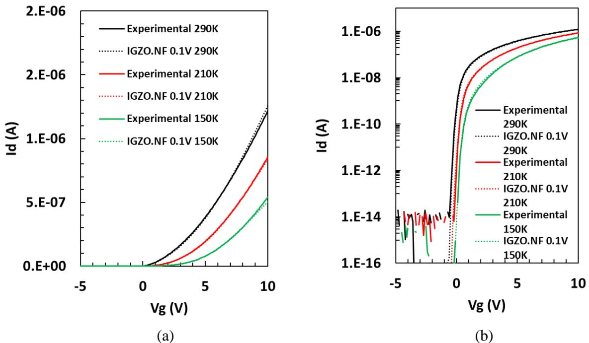
Figure 4.15: Non-Fermi mobility model with mobility as a function of temperature with  $V_D = 0.1V$ .
