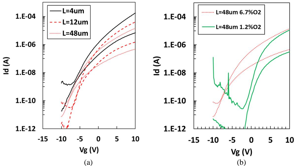
Figure 7.10: (a) Transfer characteristics of IWO TFTs, 6.7%  $O_2$ , annealed in  $O_2$  for 2 hours at 300°C, (b) Comparison of 6.7% $O_2$  annealed for 2 hours and 1.2% $O_2$  annealed for 10 hours at 300°C in dry  $O_2$
