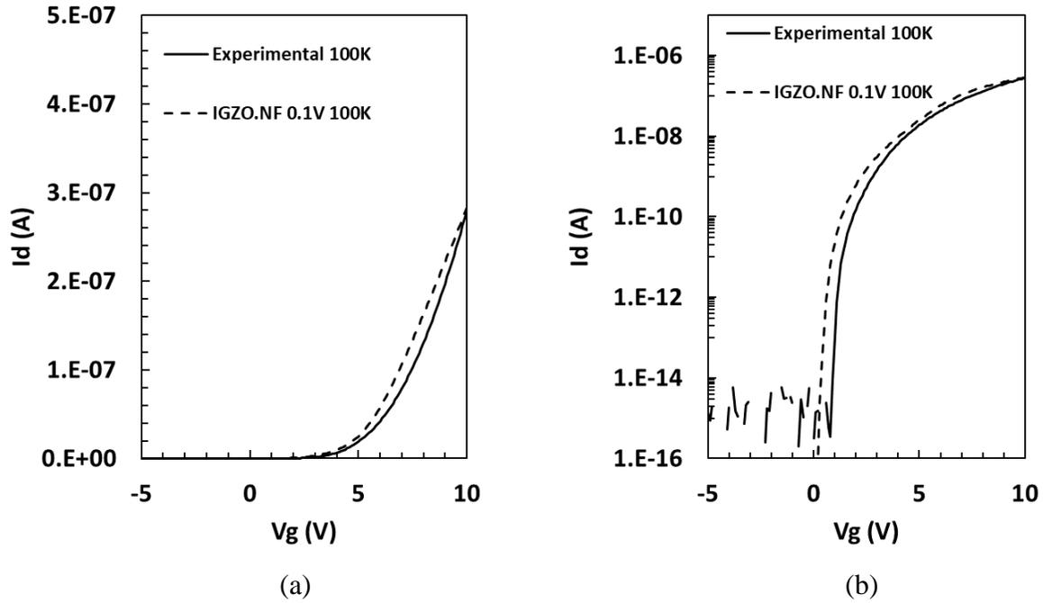
Figure 4.19: IGZO.NF model with mobility as a function of temperature at 100K in (a) linear scale and (b) Log-scale
