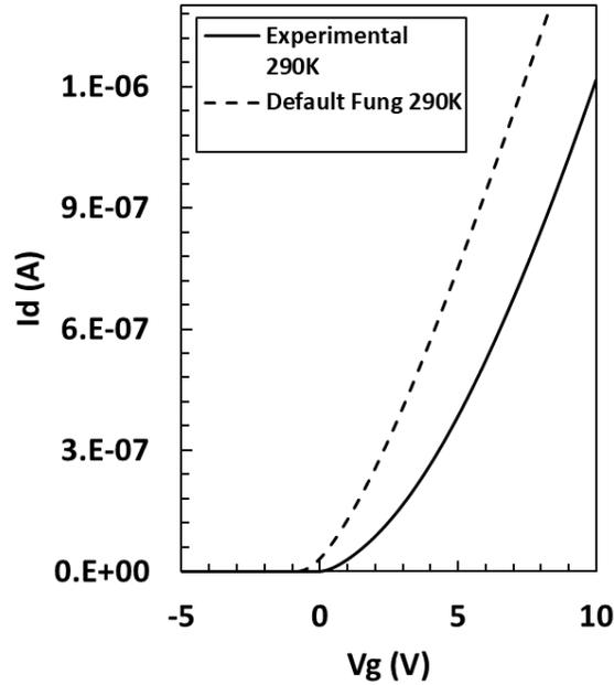
Figure 2.9: Using default Atlas IGZO parameters in Table 2-II, comparison between experimental and simulated I-V at 290K.
