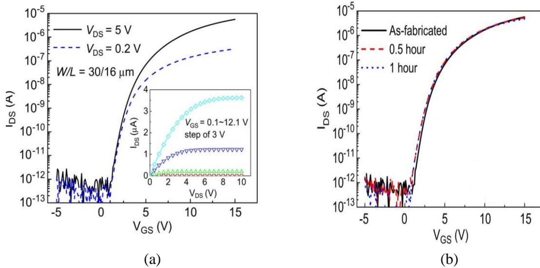
Figure 6.7: (a) Transfer and output characteristics (shown in the inset) of the self-aligned top-gate IGZO TFTs with phosphorus doped S/D regions and (b) transfer characteristics under thermal stress treatments at 200 °C. Adapted from [96].
