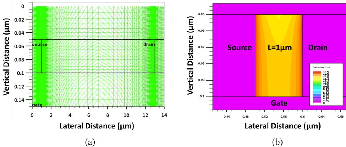
Figure 2.6: (a) Cross-section of BG TFT structure showing the mesh used for simulation. Finer mesh is used in IGZO channel and at IGZO/SiO<sub>2</sub> interface for improved accuracy. The channel length is 12 μm and gate & S/D overlap is 1 μm. (b) Electron concentration contours in IGZO channel (L=100nm, scaled for illustration only) for zero bias condition. The default defect distribution is used. Higher electron density near the S/D metal (aluminum) is due to the M-S workfunction difference.
