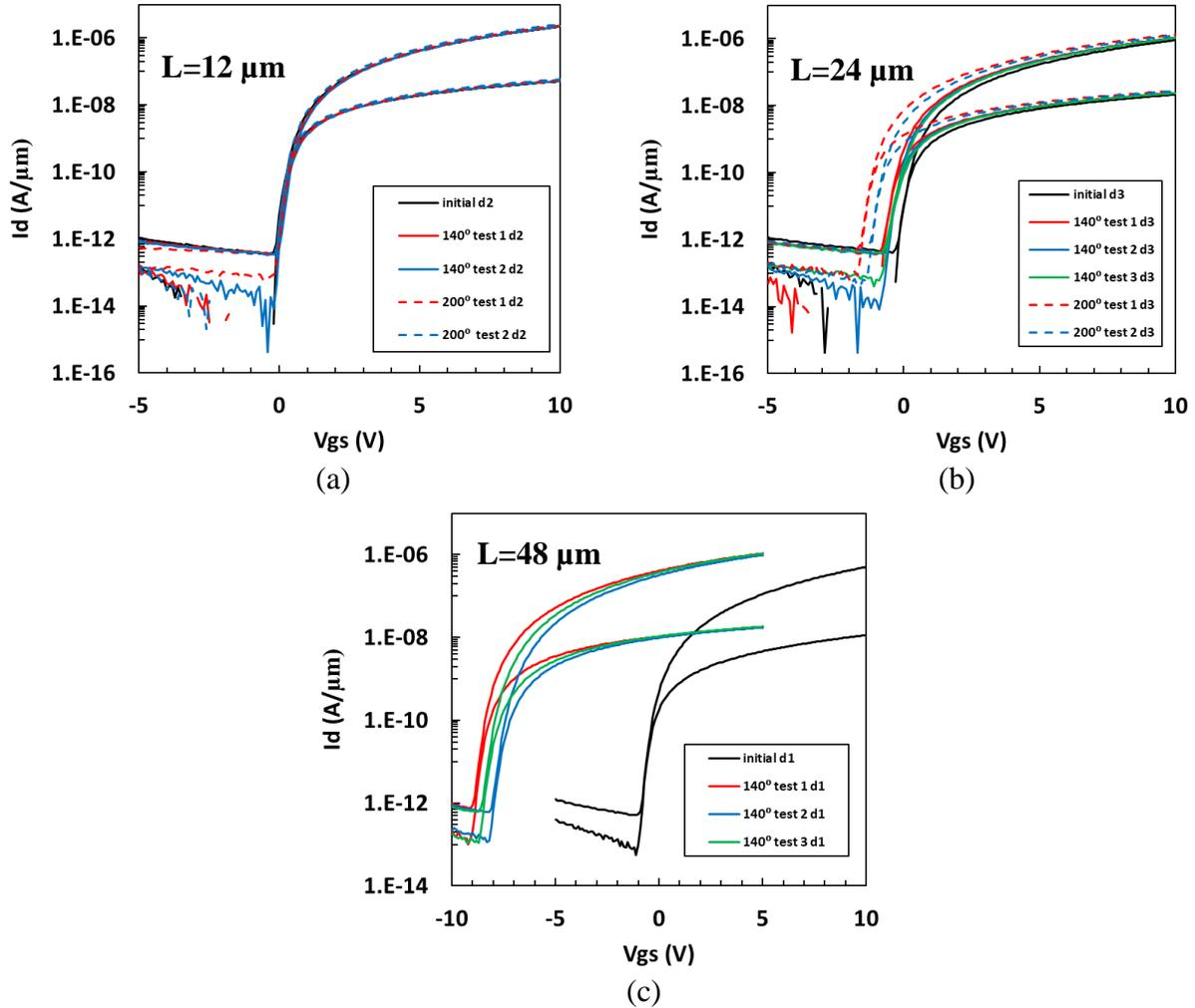
Figure 3.14: Channel length dependent behavior of ALD  $\text{Al}_2\text{O}_3$  capped DG devices with (a)  $L=12 \mu\text{m}$ , (b)  $24 \mu\text{m}$ , and (c)  $48 \mu\text{m}$  [13].
