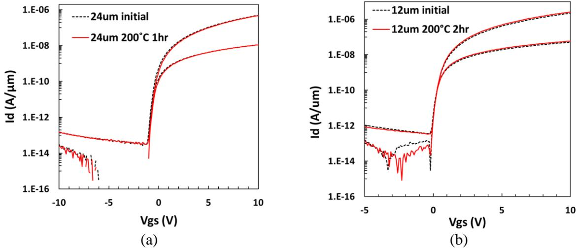
Figure 3.13: Representative characteristics of (a) BG and (b) DG devices with a 10 nm ALD  $\text{Al}_2\text{O}_3$  capping layer deposited at 200 °C above the back-channel passivation/gate oxide. Channel length values are indicated [13].
