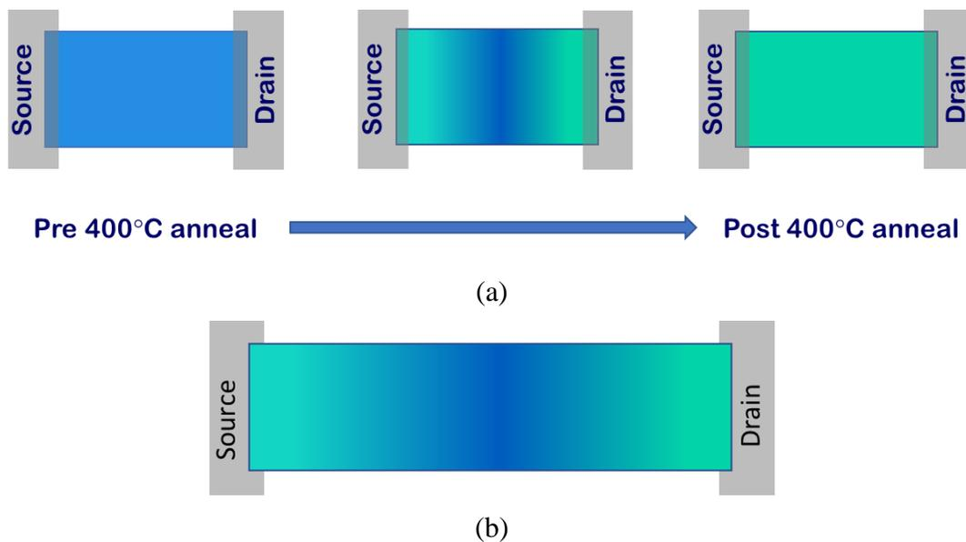
Figure 3.15: (a) Water segregation from channel due to source/drain electrodes acting as a getter. Blue regions indicate the presence of H<sub>2</sub>O molecules. (b) In longer channel devices the water is not effectively gettered during subsequent anneal.
