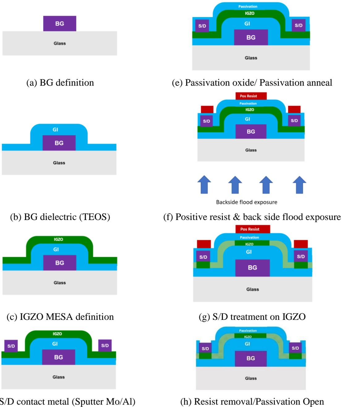
Figure 6.19: Step by step cross-sectional schematic of SA-BG device, where the textured and non-textured IGZO represents implanted and non-implanted regions, respectively. Note that in this process scheme the implant is blocked in both channel and S/D metal contact regions.
