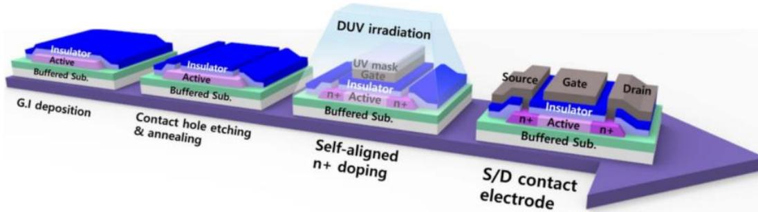
Figure 6.2: Schematic process flowchart for a coplanar SA-TG IGZO TFT with S/D regions formed by DUV irradiation energy of  $30 \text{ J/cm}^2$ . Adapted from [92].
