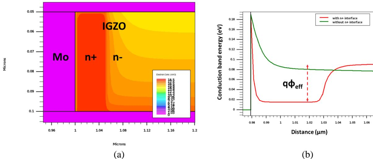
Figure 4.20: (a) n+ interface region (50 nm) at the source end with the oxygen-vacancy donor concentration increased to  $N_{OV}=10^{20} \text{ cm}^{-3} \text{ eV}^{-1}$ , (b) n+ interface region near the source narrows the tunneling barrier and effectively reduces the barrier height ( $q\phi_{eff}$ ) for source injection.
