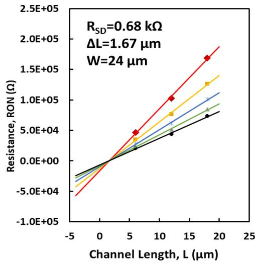
Figure 6.14: T-M analysis for  $^{40}\text{Ar}^+$  implanted SA-TG devices using channel length of 6, 12, 18  $\mu\text{m}$  devices. The resistance is calculated at  $V_g = 2, 4, 6, 8, 10 \text{ V}$  with drain voltage at  $0.1 \text{ V}$ . The extracted parameters are  $\Delta L = 1.67 \mu\text{m}$  and  $R_{SD} = 0.68 \text{ k}\Omega$  for  $24 \mu\text{m}$  wide device.
