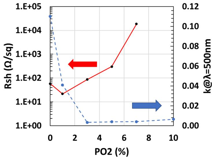
Figure 7.15: Sheet resistance &  $k@λ=500nm$  as a function of oxygen partial pressure during sputter of ITGO film, note that for  $P_{O_2}=10\%$  the  $R_{sh}$  was not measurable.
