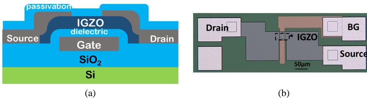
Figure 2.1: (a) Cross-section schematic of a passivated BG TFT, unpassivated BG device does not have the passivation on top, (b) top-down view of the fabricated BG device
