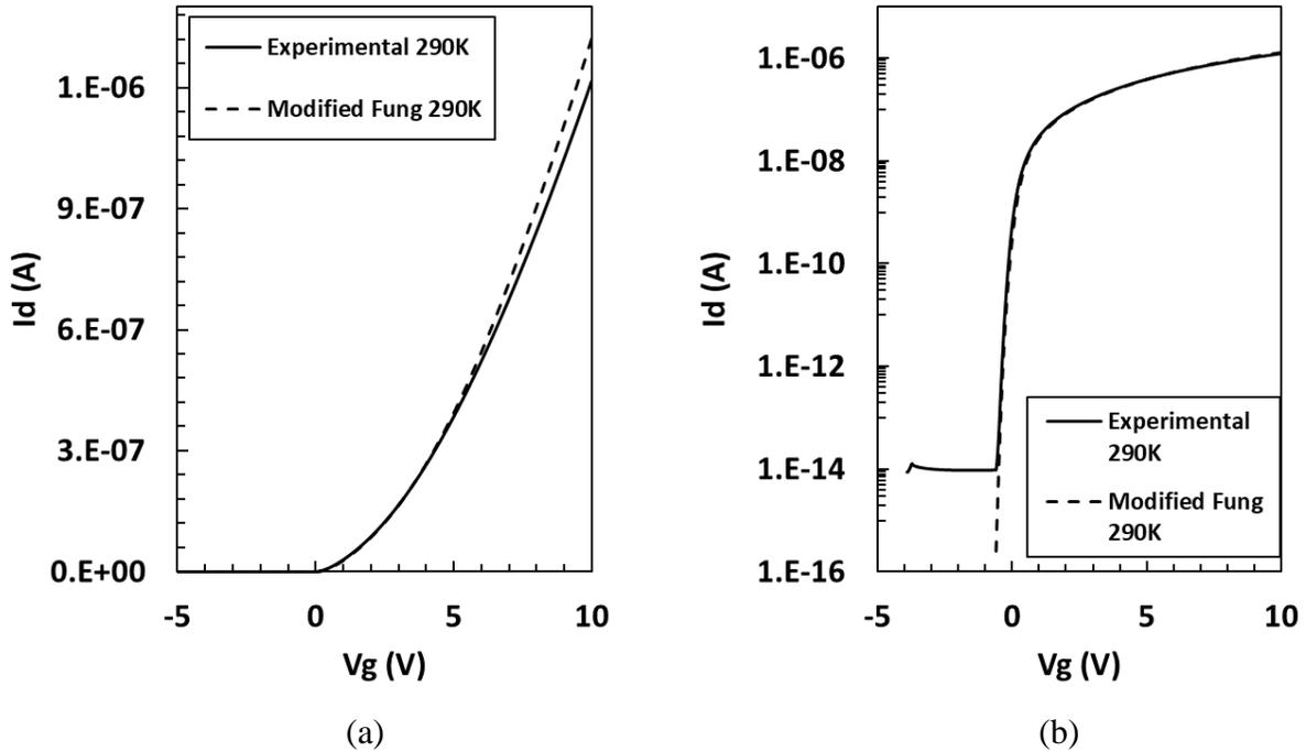
Figure 2.10: Comparison of experimental vs simulated passivated I-V with using modified passivated parameters from Table 2-III.
