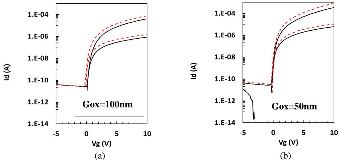
Figure 5.9: Devices fabricated on Corning NXT glass substrate with (a) 100 nm and (b) 50 nm gate oxide respectively. In (a) solid line represents  $L=6 \mu\text{m}$  and dashed line  $L=4 \mu\text{m}$  and in (b) solid line represents  $L=2 \mu\text{m}$  and dashed line  $L=1 \mu\text{m}$ .
