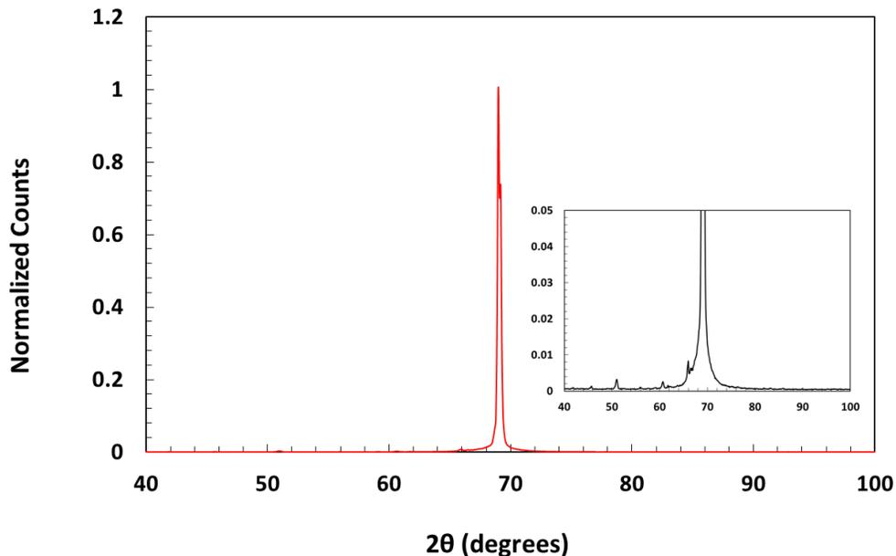
Figure 7.6: XRD spectrum of annealed IWO film for 2hr in  $O_2$  at  $400^\circ\text{C}$  on a silicon wafer. The peak at  $\sim 70^\circ$  is from the Si wafer used as substrate, absence of any additional peak confirms the amorphous nature of the annealed films. The inset is a zoomed plot to show the noise margin.
