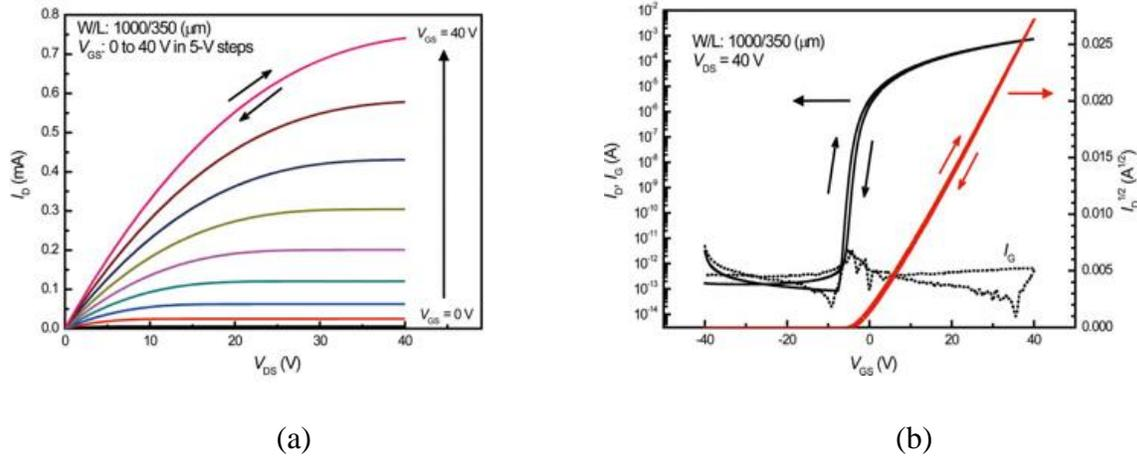
Figure 7.2: IWO TFT (a) family of curves and (b) transfer curves, with  $\mu_{FE} = 19.3 \text{ cm}^2/\text{V}\cdot\text{s}$ ,  $I_{ON}/I_{OFF} = 8.9 \times 10^9$ , and  $SS = 0.47 \text{ V/decade}$  [107]
