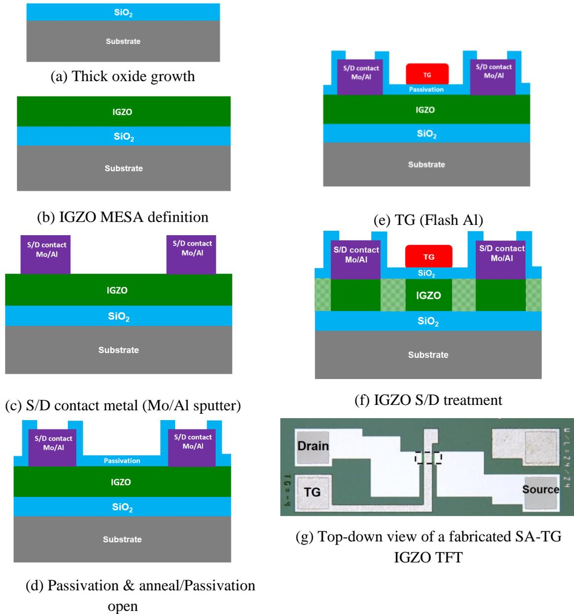
Figure 6.9: (a-f) Step by step cross-sectional schematic of SA-TG (Type-TL (Treatment Last)) device, where the textured and non-textured IGZO represents implanted and non-implanted regions, respectively. Note that in this process scheme (type-TL) the implant is blocked in both channel and S/D metal contact regions and (g) top-down view of a fabricated SA-TG IGZO TFT.
