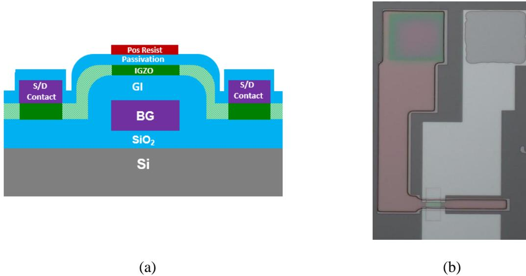
Figure 6.17: (a) Cross-sectional schematic and (b) top-down view of pseudo-SA BG device, where the textured and non-textured IGZO represents implanted and non-implanted regions, respectively. Note that in this process scheme, the implant is blocked in the channel region only and the alignment of the BG pattern is critical.
