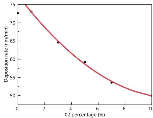
Figure 7.13: ITGO deposition rate with oxygen partial pressure during sputter
