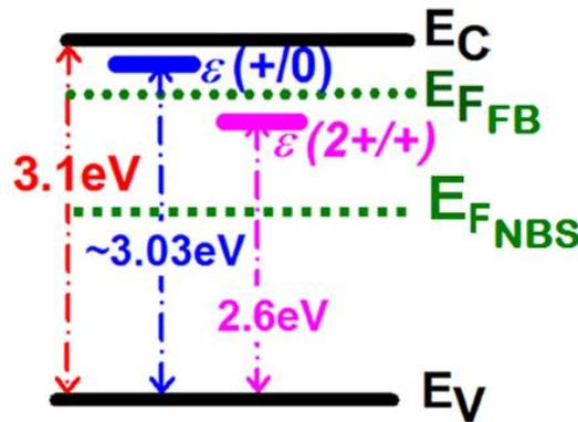
Figure 3.19: IGZO energy band diagram, showing single-donor ( $V_O^+$ ) and double-donor ( $V_O^{2+}$ ) oxygen vacancy defect states within the bandgap. The Fermi Energy ( $E_F$ ) is approximated at flatband and NBS conditions. Using the indicated energy differences referenced to  $E_V$ , the energy levels for the  $V_O^+$  and  $V_O^{2+}$  states are calculated to be 70 meV and 500 meV below  $E_C$ , respectively. Figure adapted from Chowdhury et al. [62].
