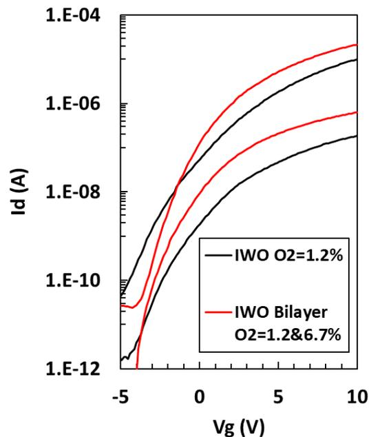
Figure 7.11: IWO TFTs with  $L=48$   $\mu\text{m}$  employing bilayer structure of oxygen content in the channel showing improved I-V characteristics over a single layer channel.
