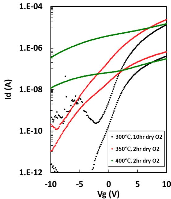
Figure 7.9: Transfer curve of 24um device sputtered in ambient of 1.2%O<sub>2</sub> and annealed at different temperatures.
