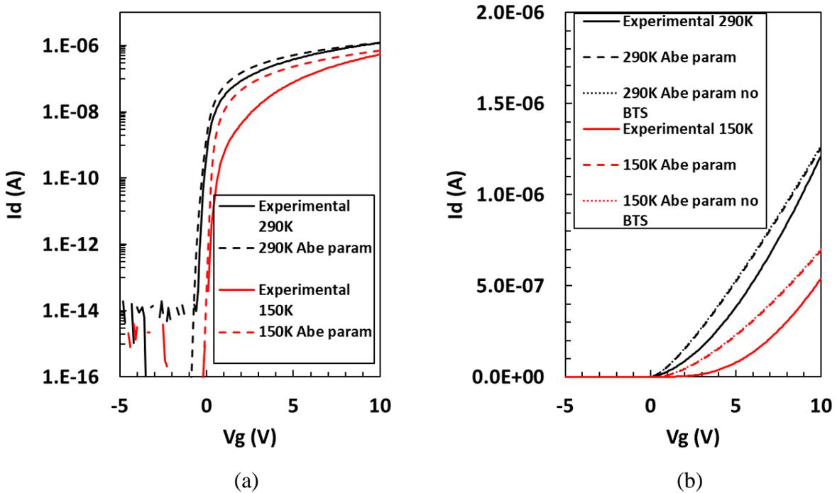
Figure 4.13: (a) Experimental results with simulated I-V using Abe's parameters (Table 4-II, column 2), (b) Simulated I-V with or without Abe's BTS values showing no effect on the device behavior.
