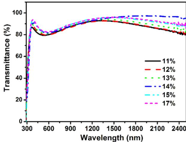
Figure 7.1: Optical transmittance spectra of IWO films with different  $O_2/Ar$  ratios [111]
