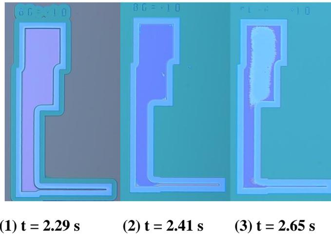
Figure 6.28. Photoresist-coated BG structures that were flood exposed for times indicated; all samples exhibit significant edge exclusion. The short exposure time of sample#1 did not clear the field region, whereas the long exposure time of sample #3 resulted in partial clearing of photoresist over the planar BG region [99].
