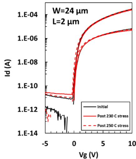
Figure 5.7: BG devices with ALD  $\text{Al}_2\text{O}_3$  capping layer deposited at  $200^\circ\text{C}$  with scaled channel lengths and 1-hour sequential thermal stress treatment temperatures as indicated [26].
