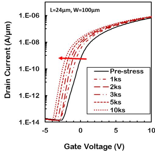
Figure 3.18: I-V characteristics of  $L/W=24/100$   $\mu\text{m}$  device showing a significant left shift in  $V_T$  under NBS [40].
