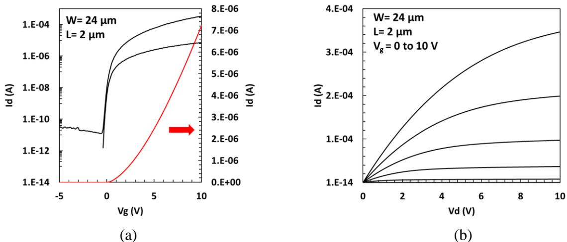
Figure 5.5: Transfer characteristics (a) and output characteristics (b) of a representative BG device with  $2\ \mu\text{m}$  channel length. The Y2 axis in (a) shows the low-drain bias measurement on a linear-scale, demonstrating the influence of band-tail states on electrical behavior [58].
