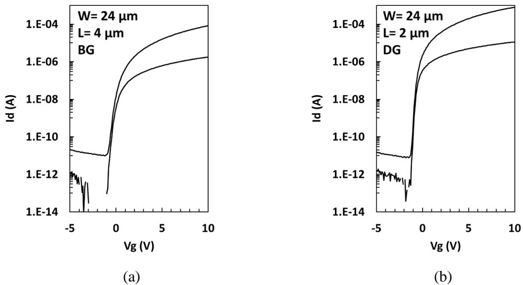
Figure 5.2: Transfer characteristics of IGZO TFTs with 100 nm  $\text{SiO}_2$  gate/passivation dielectric. Drain bias conditions are 0.1V and 10V, (a) BG configuration with  $L = 4 \mu\text{m}$ . (b) DG configuration with  $L = 2 \mu\text{m}$  [58].
