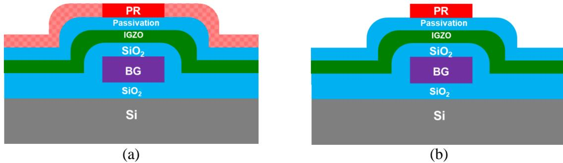
Figure 6.27: Cross-sectional schematic of a SA-BG lithographic process (a) after exposure and (b) after develop [99].
