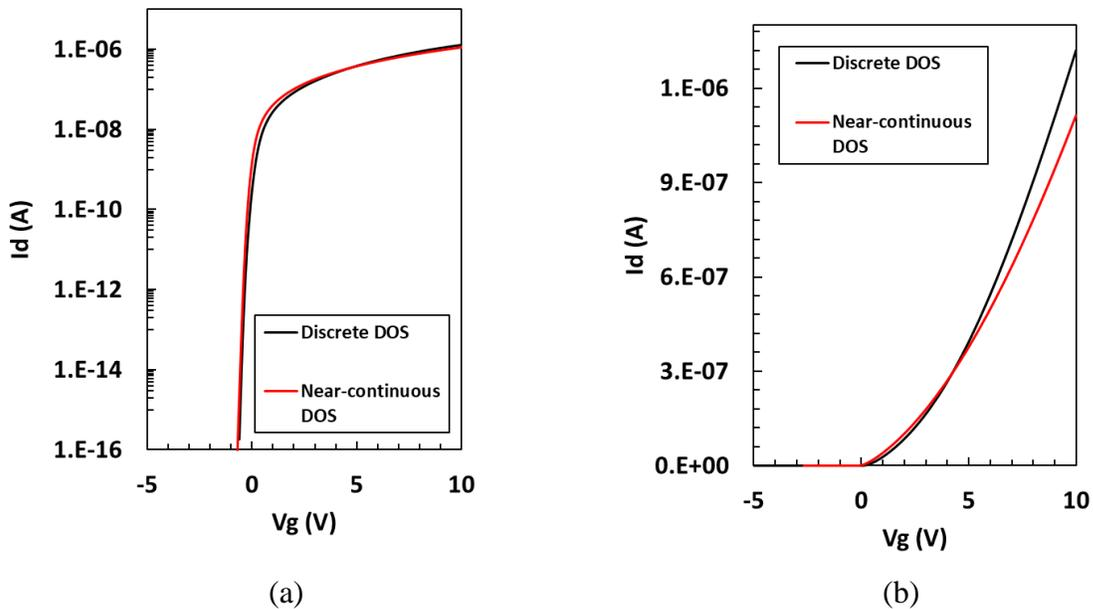
Figure 2.5: Comparison of simulated electrical characteristics with number of discrete levels in (a) log scale and (b) linear scale. Although there is negligible difference, the discrete DOS is used hereafter to minimize run-time.
