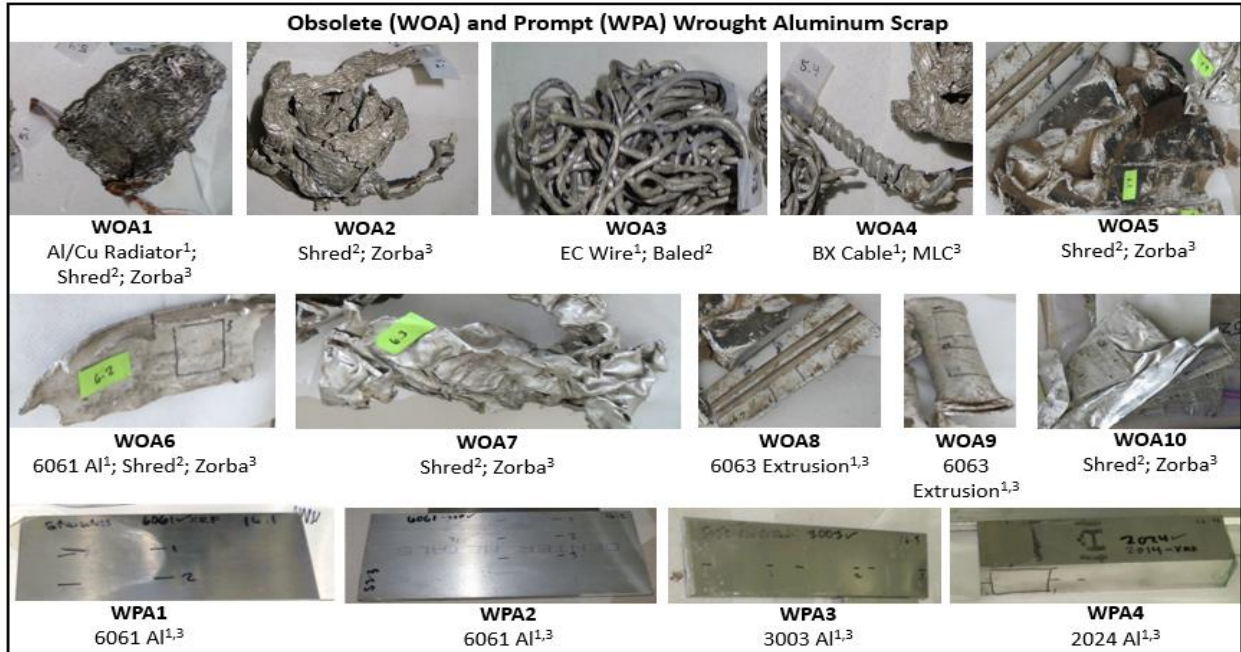
Figure 3.5 Above are the wrought obsolete (WOA: first two rows) and prompt (WPA: third row) scrap samples evaluated in this section; sample IDs are referenced below each image. Descriptors below the ID number are based off the condition of image and demonstrate the variety of ways the metal could be sorted. Superscripts indicate the following: original product 1 ; how it will be processed 2 (or how it was processed prior to our collection of the sample); likely commodity grouped with 3 . Superscripts “2” and “3” depend on volume and equipment; if a “2” is not present, that means no processing required.
