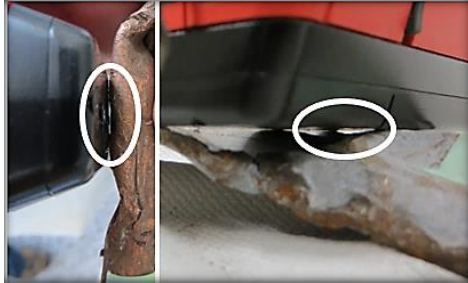
Figure 3.3 Small gaps between the surface of the detector and the sample, such as the ones circled in white above, prevented the instrument from taking readings.
