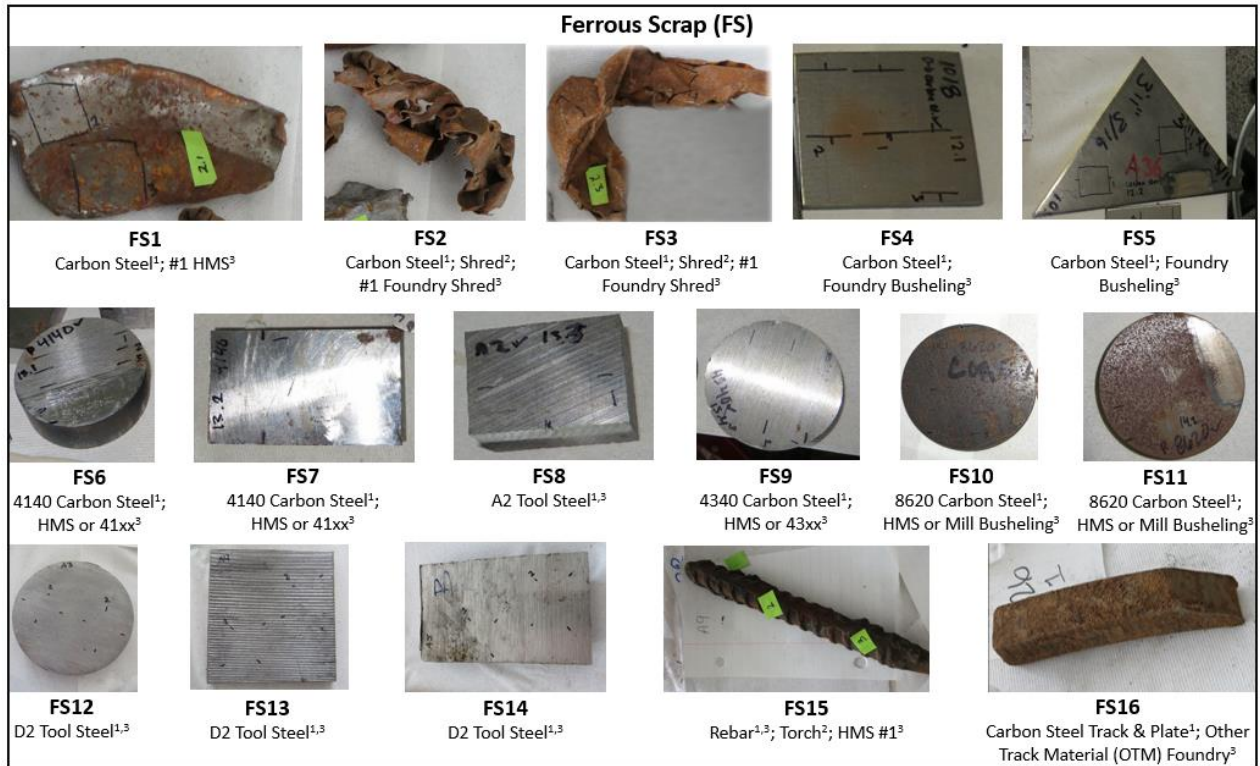
Figure 3.4. Ferrous scrap includes a variety of iron (Fe), carbide steel, tool steel, rebar, and plate and structural. Above is the assortment of ferrous scrap reviewed for this study with the sample ID numbers referenced below each image. Descriptors below the ID number are based off the condition of image and demonstrate the variety of ways the metal could be sorted. Superscripts indicate the following: original product 1 ; how it will be processed 2 (or how it was processed prior to our collection of the sample); likely commodity grouped with 3 . Superscripts “2” and “3” depend on volume and equipment; if a “2” is not present, that means no processing required.
