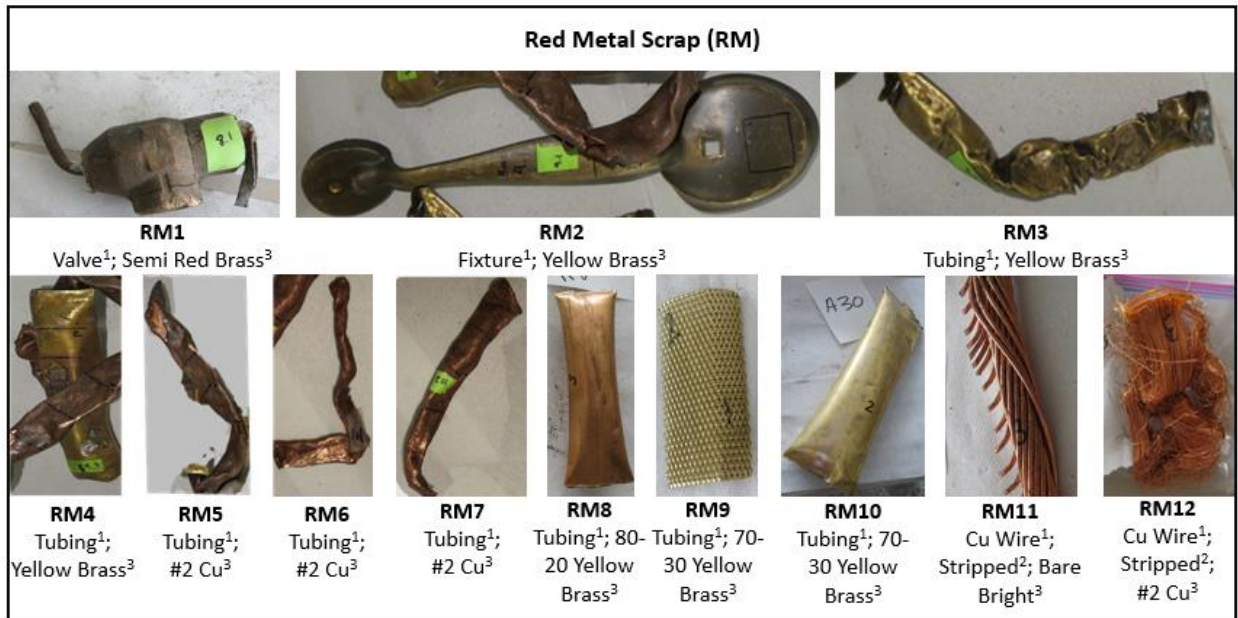
Figure 3.12 Red metals include copper, brass (red and yellow), and bronze. The red metal scrap evaluated in this study can be found above with sample ID numbers indicated below each image. Sample ID numbers are accompanied by descriptors below (based off the condition of the image) and demonstrate the variety of ways the metal could be sorted. Superscripts indicate the following: original product 1 ; how it will be processed 2 (or how it was processed prior to our collection of the sample); likely commodity grouped with 3 . Superscripts “2” and “3” depend on volume and equipment; if a “2” is not present, that means no processing required.
