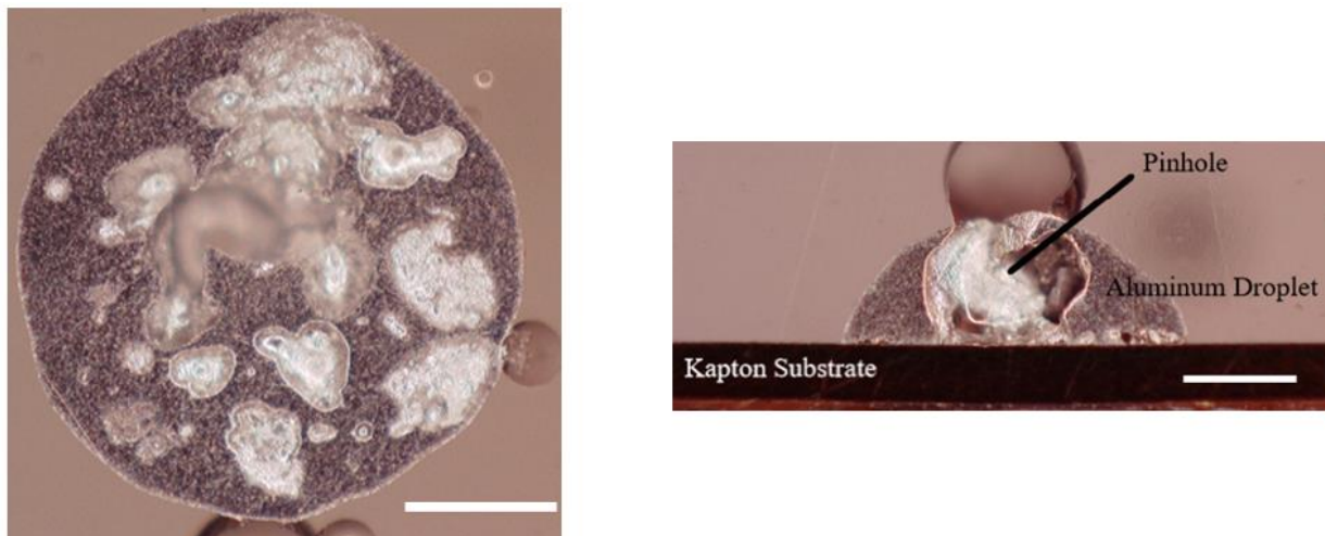
Figure 5.3: (a) Bottom view of a printed droplet (b) Side view of the droplet cross-section. Scale bar = 250 \mu\text{m} .
