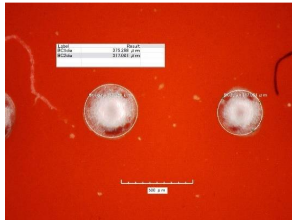
Figure 4.1: Microscopic image of droplet diameter being measured on the Hirox microscope.
