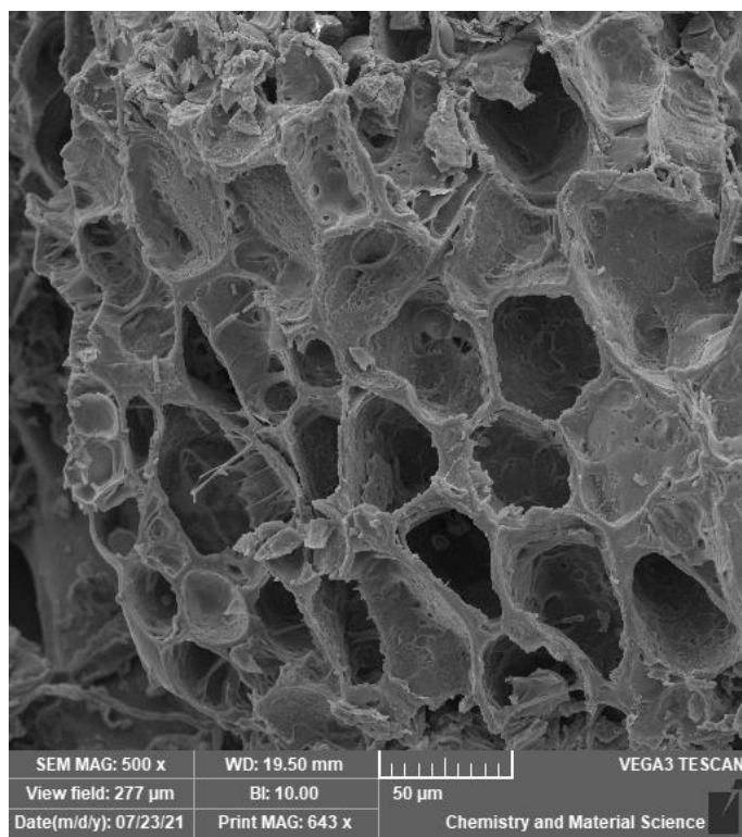
Figure 5. SEM image of pores seen on food waste biochar at 500X magnification.
