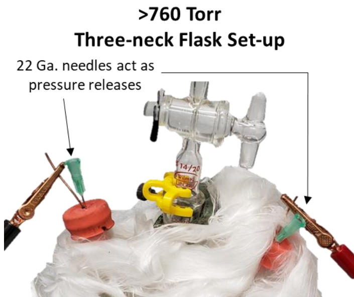
Figure 26 Picture of the three-neck flask set-up used for Joule-heating driven CVD, with 22 Ga. needles inserted into the outer necks' rubber septa to act as pressure releases.
