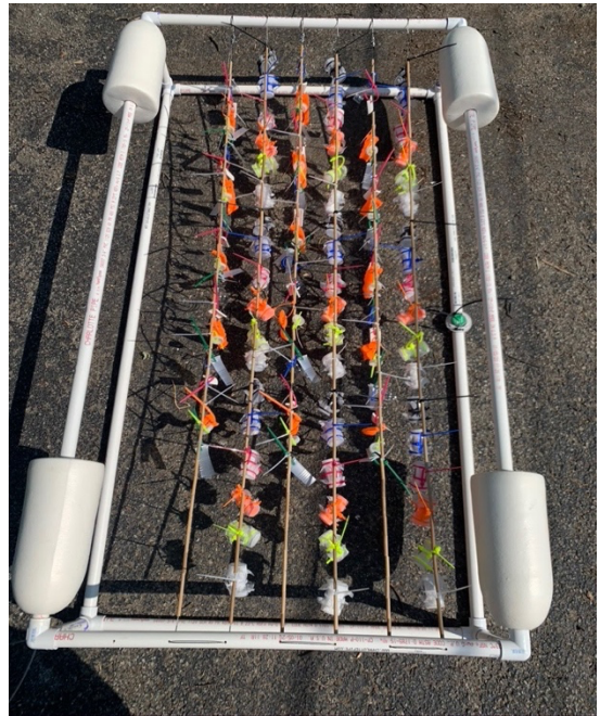
Figure 3.2. Completed surface water raft used in field aging experiments
