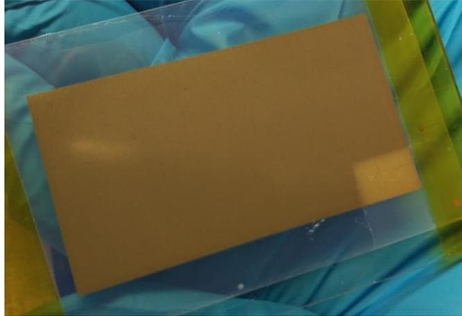
**Figure 6.3** A single-electrode printed device used for droplet ejection.<sup>37</sup>
