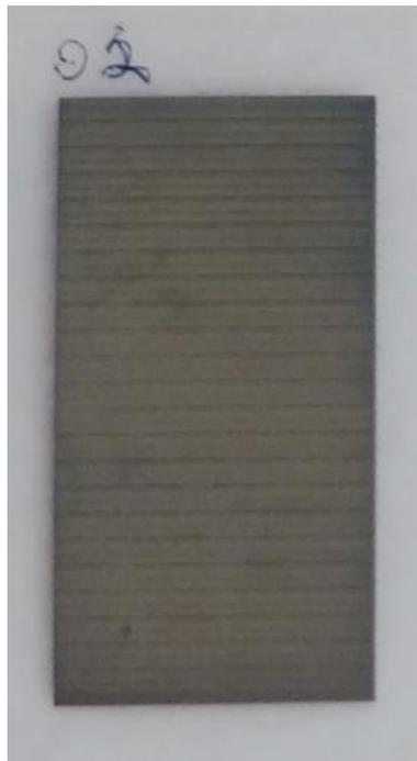
**Figure 6.1** An early inkjet-printed electrode.
