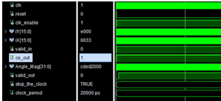
Figure 5.29: CORDIC Testbench Waveforms.
