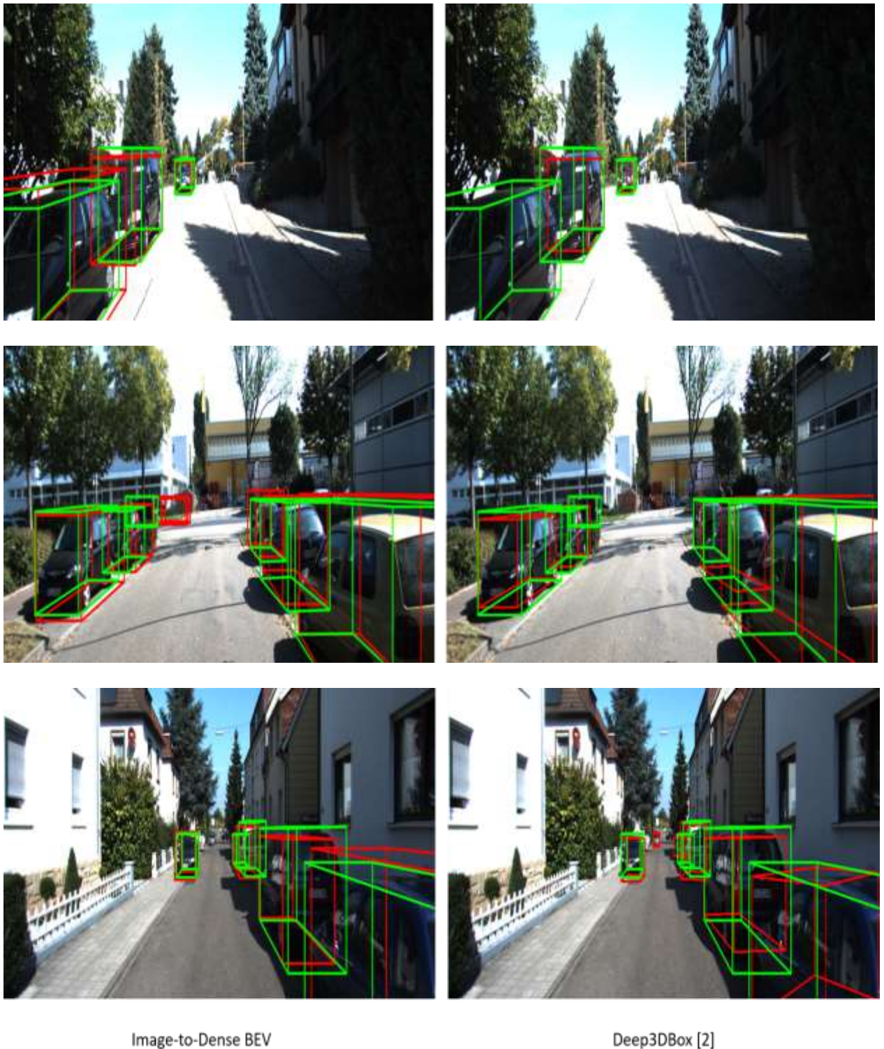
Figure 5.5: Qualitative comparison of our 3DOD model trained on dense BEV predicted images (left) and the Deep3DBox [2] method (right). Predicted boxes are in red and ground truth boxes are in green.
