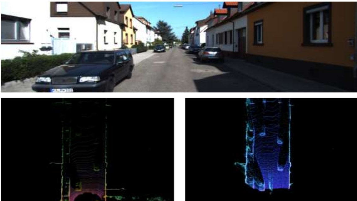
Figure 3.4: Sparse BEV (left) and dense BEV (right) image projection of a sample image (top) from the KITTI dataset.
