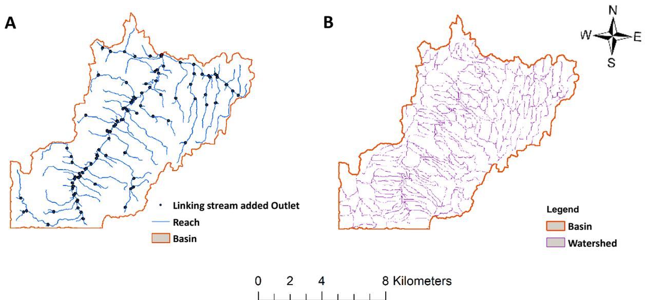
Figure 6: Watershed Delineation in SWAT model (A) Stream networks and monitoring points, (B) Sub-basins definition of SWAT.
