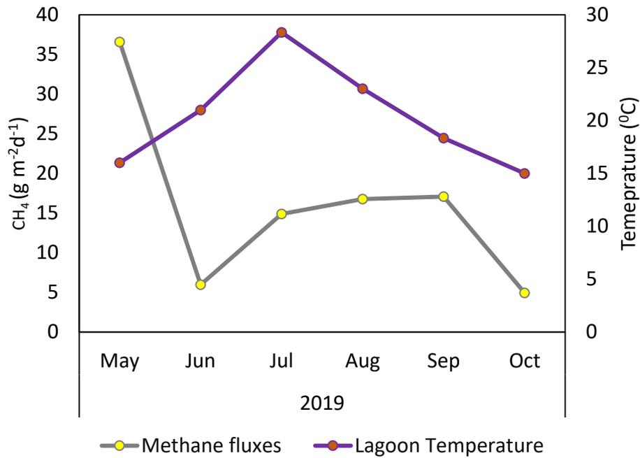
Figure B.2: Mean daily fluxes of methane (in g CH<sub>4</sub> m<sup>-2</sup>d<sup>-1</sup>) and lagoon surface temperature (°C).
