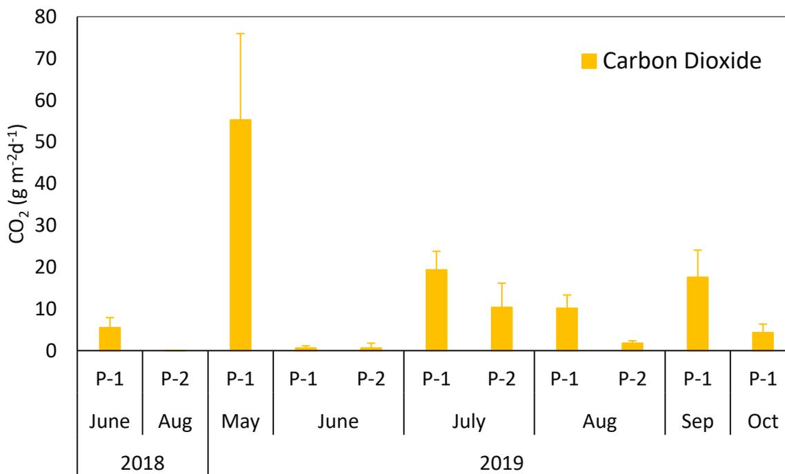
Figure B.1: Mean daily release of methane (mean +/- SE) (top panel), carbon dioxide (bottom panel). Emission of GHG from digestate storage ponds during the summers of 2018 and summers and falls in 2019.
