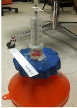
*Figure A.5: Gas trap designed to measure GHG emissions from digestate storage pond.*
