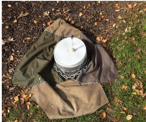
*Figure A.7: Soil chambers for flux measurements*
