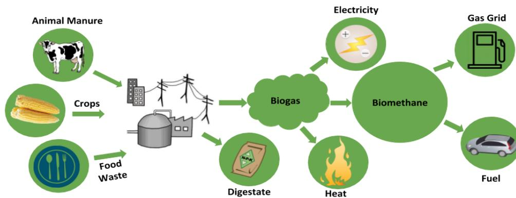
Figure 1: Schematic diagram of Anaerobic Co-Digestion (AcoD) Process.
