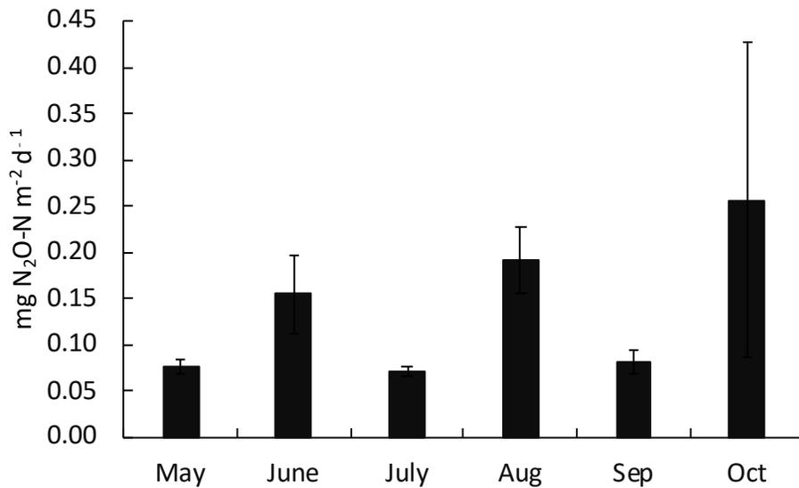
Figure 7: Daily release of nitrous oxide (mean +/- SE) from the two primary storage ponds at the digester facility measured using gas traps in 2019 (n=4 for each pond).
