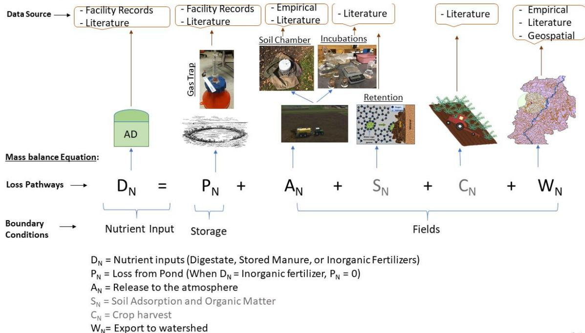
Figure 4: Nitrogen mass balance approach to understand the potential ecological impacts of food waste digestate management, showing each potential loss pathway and indicating the source of data used to parameterize the model: empirical measurements, literature review, facility records, and geospatial model predictions. Values in gray text were not included in the mass balance model.
