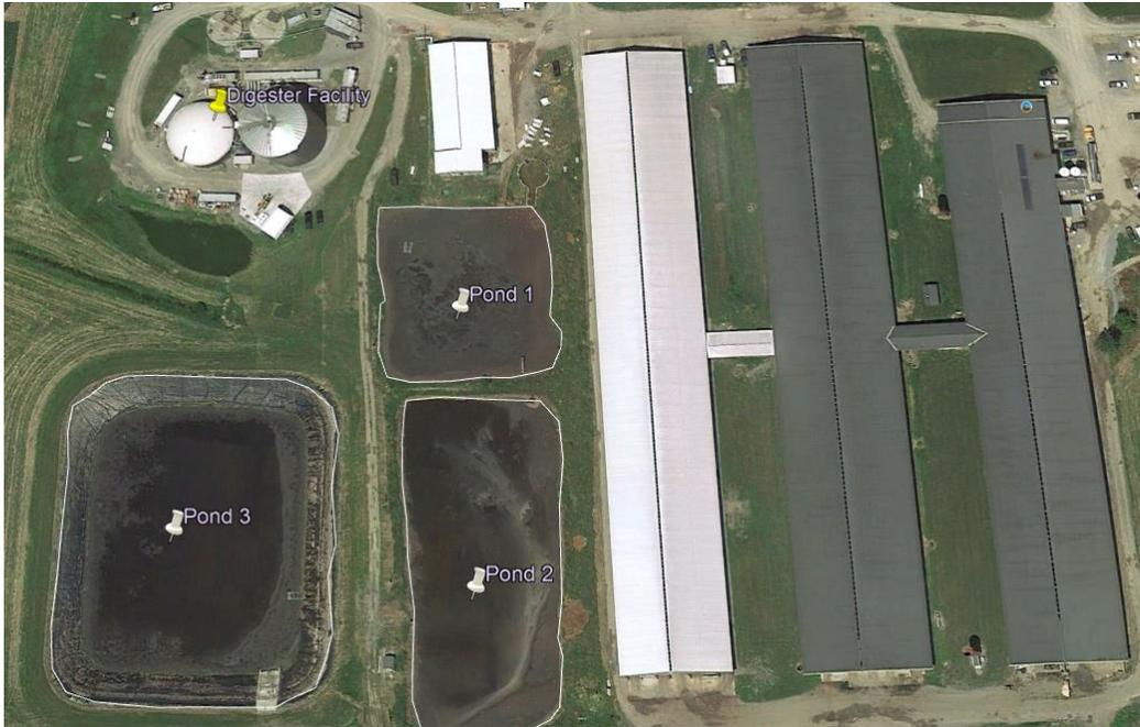
Figure A.3: Digester facility, illustrating the location of the three digestate storage ponds.
