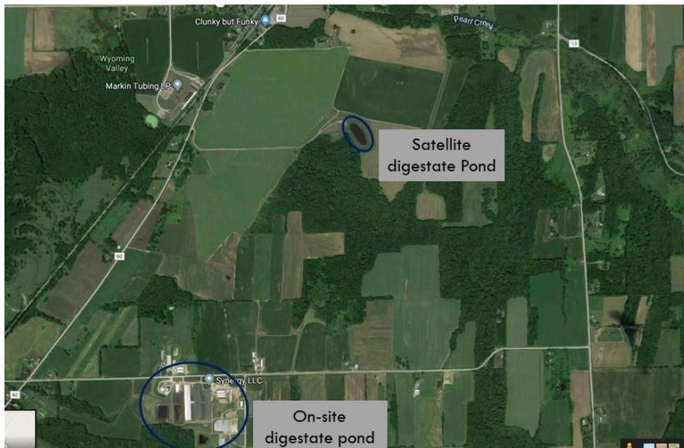
Figure A.4: On-site and satellite digestate storage ponds.
