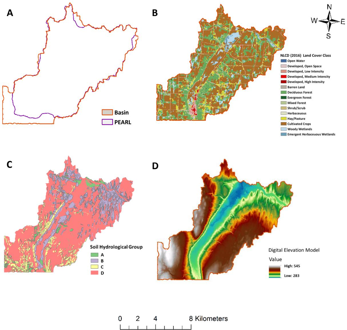
Figure 5: Input parameters for the SWAT model include (A) Boundary of Pearl Oatka watershed and SWAT basin, (B) land use land cover, (C) soils groups, and (D) the slope percent.
