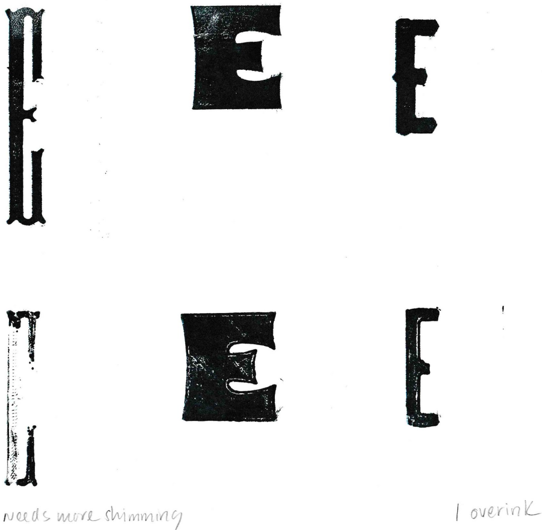
Figure 18: First test print of facsimiles. The first test print of the facsimiles was overinked. It was determined that the 3D printed Antique Tuscan (bottom left) needed more shimming to help achieve a better imprint. Scan courtesy of the author.
