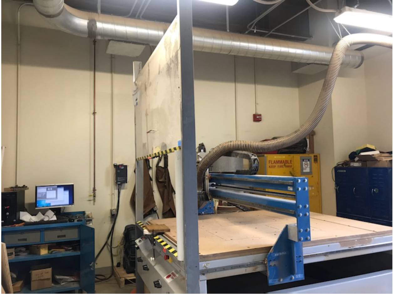
Figure 15: CNC router. The image is of the CNC router at RIT's Construct that was used to create the wooden facsimiles in this project. Image courtesy of Juilee Decker.
