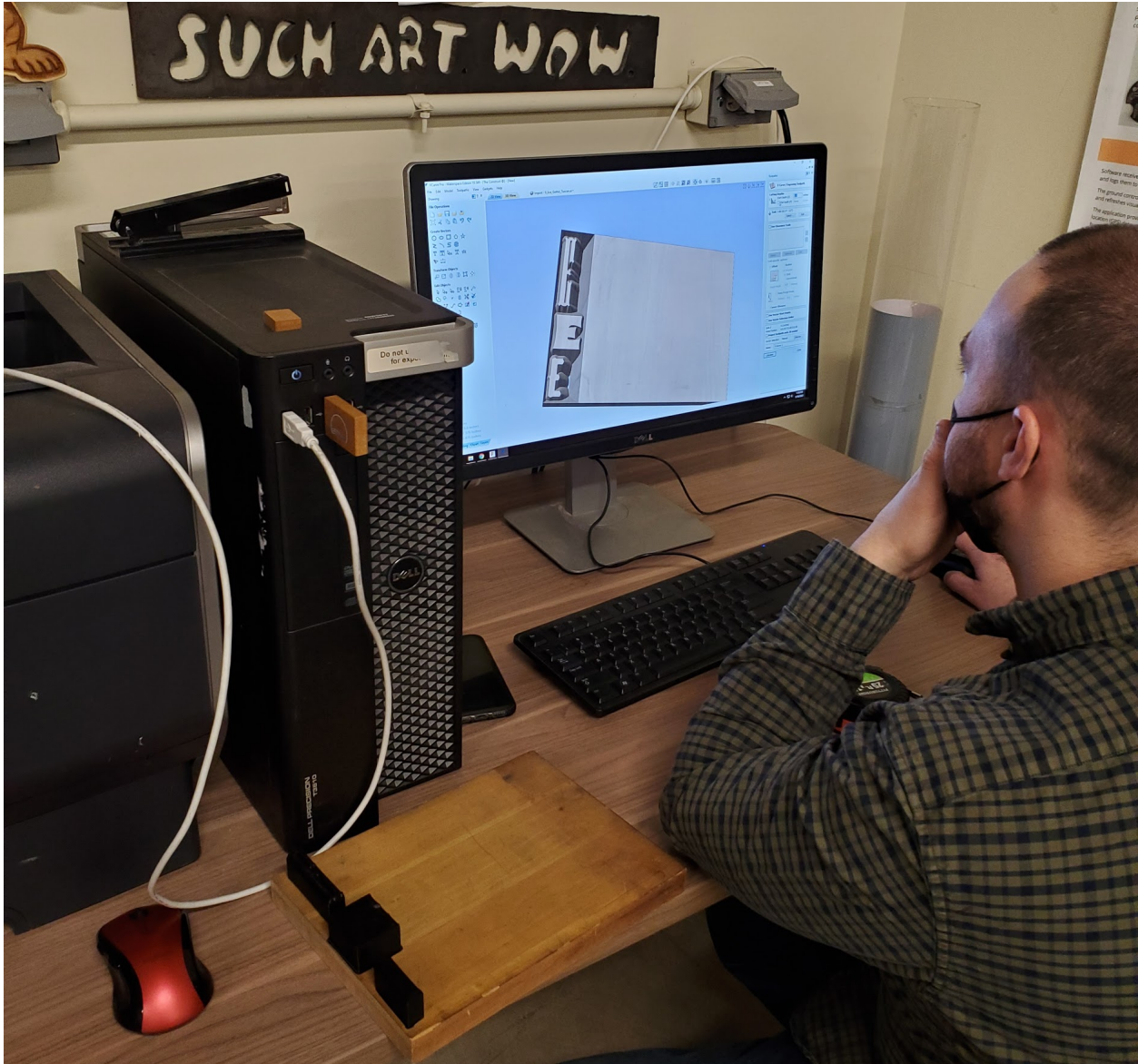
Figure 14: Mike Buffalin adjusting the vector files in VCarve. The image shows Mike Buffalin, RIT Construct, adjusting the size of the vector files of three fonts and the depth that the router would carve at. Image courtesy of the author.
