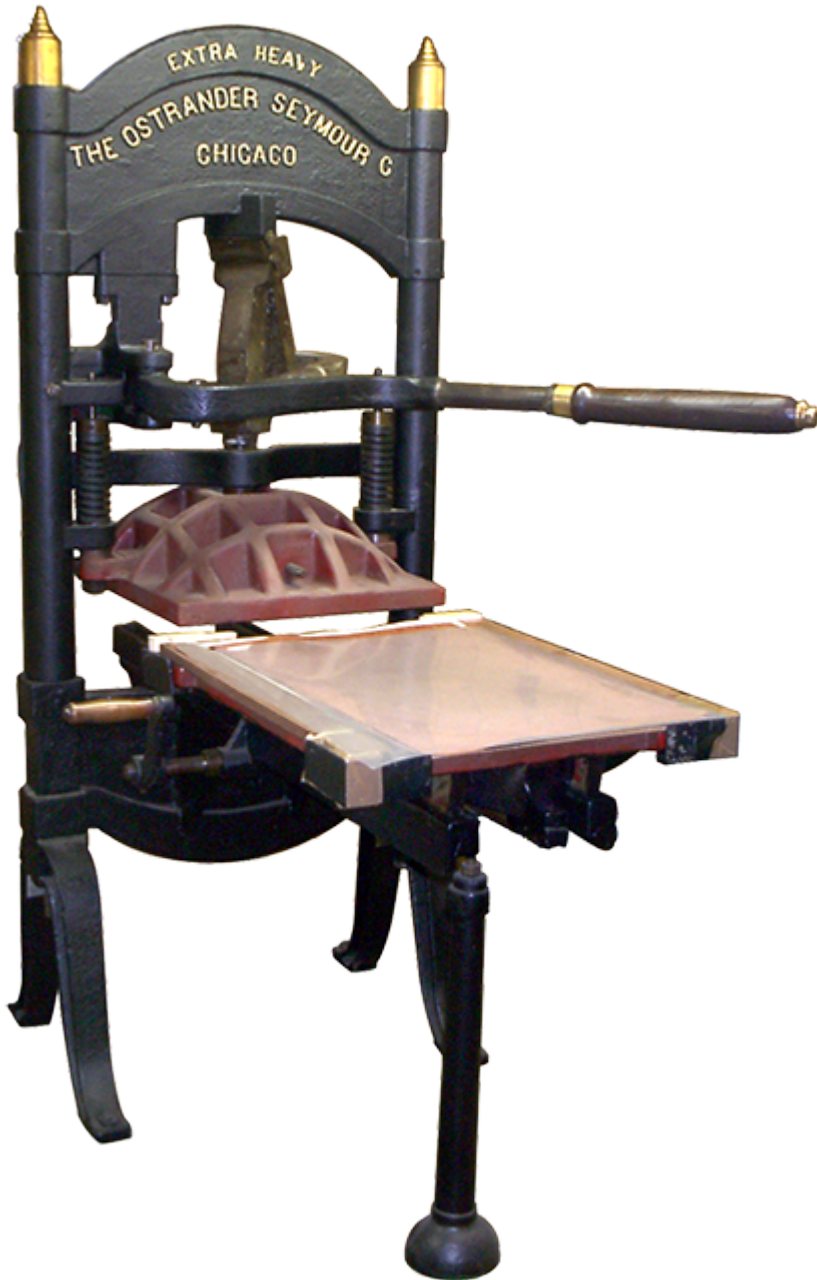
Figure 1: A Washington Printing Press. This is one of many models of the Washington Printing Press that utilizes the figure four toggle as its printing mechanism. Press, Briar. "Washington." Letterpress Commons.
