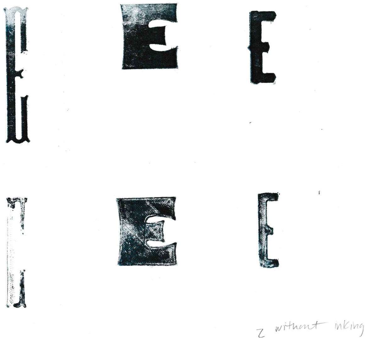
Figure 19: Second test print of facsimiles. The image shows the second test print which was performed to remove excess ink from the typeface before adding additional shimming to the facsimile in the bottom left. Scan courtesy of author.
