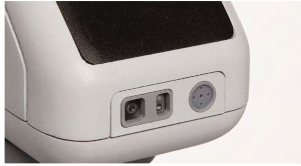
Fig 8.3: lidar sensor and RGB camera
