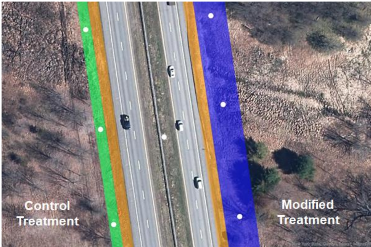
Figure 2: A visual representation of the treatment design at each site. The orange strip on both sides of the road indicates the ~5m safety strip that is required to be mowed by regulation. The blue represents the modified mowing pattern that is wider and mowed less frequently than the control mowing pattern, as seen in green.
