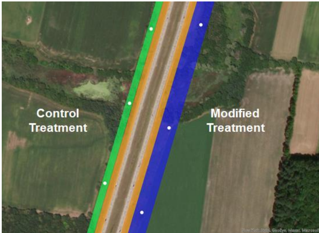
Figure 2: A diagram of the mowing treatment at each site. The strip on both sides of the road, as seen in orange, depicts the 15 ft safety strip that is mowed for safety purposes. The green represents the control mowing pattern and blue represents the later and wider, modified mowing pattern.
