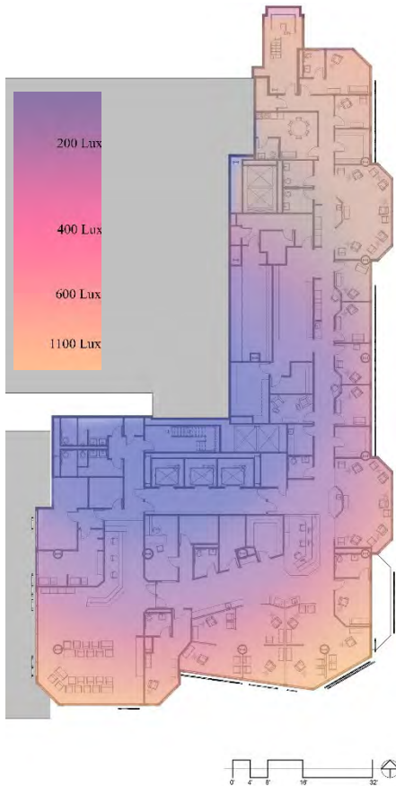
Figure 18 - Daylighting Analysis At Summer Solstice Designed By Author.
