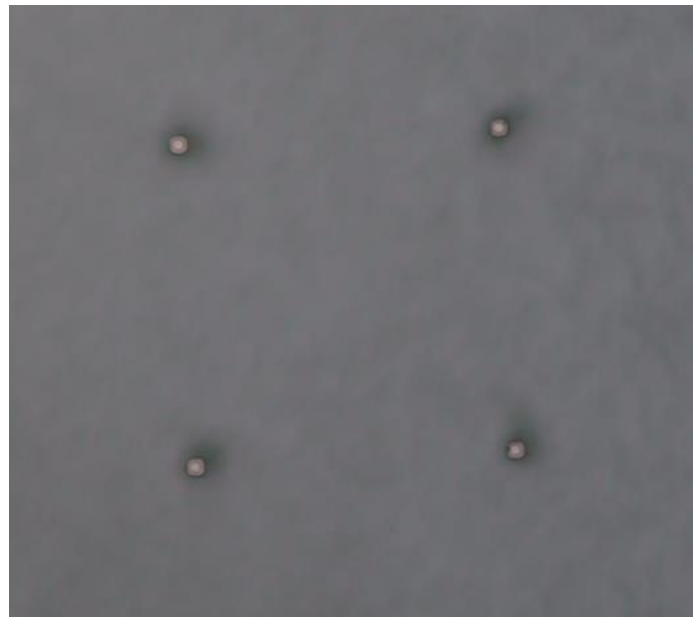
Figure 7.3: Microscope image of re-metallized tips.
