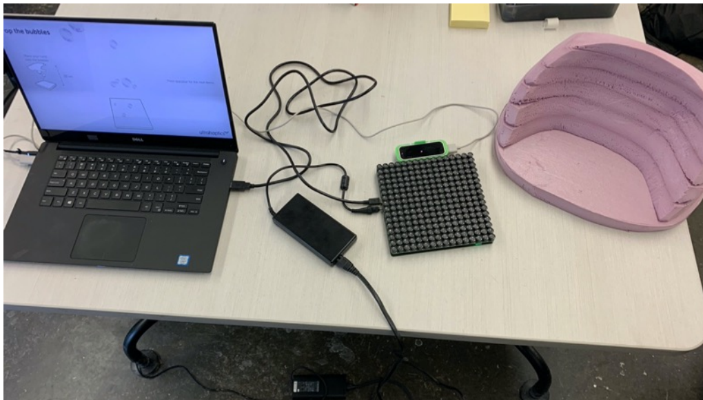
fig. 4 – Haptic development unit in center of photograph, foam scale model to the right.
