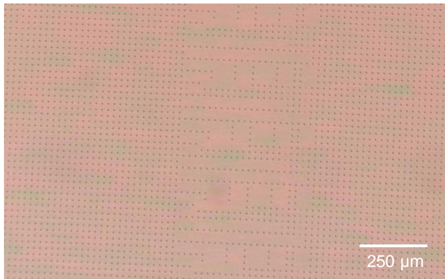
Fig. 39 Improved pattern uniformity with use of the plastic spacer and vacuum.
