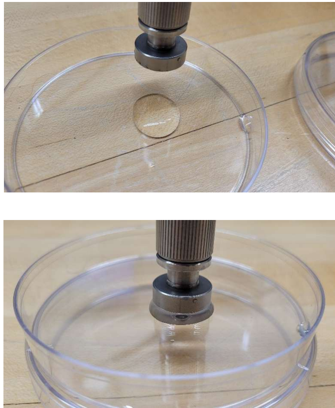
Figure 3.5. Phantom Measurement Setup with Dielectric Probe
