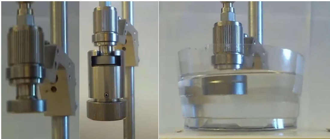
Figure 3.3. Free Space, Short and Water Calibration Steps
