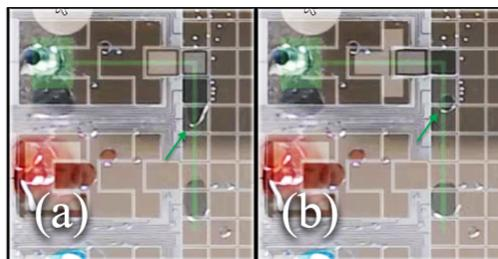
**Figure 6.35:** Image sequence from the second automated droplet transport and extraction protocol where a droplet is spontaneously created from a random pinning point on the device surface
