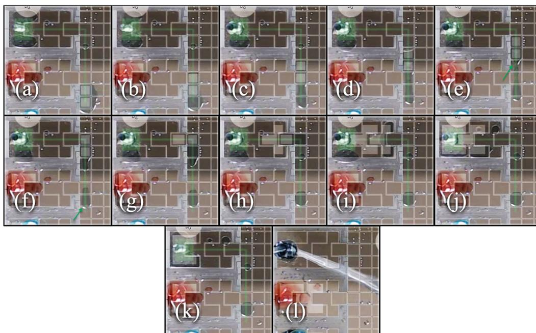
**Figure 5.28:** Image sequence from an automated droplet transport and extraction protocol using DNA brick 1 (red) and brick 2 (blue) on the final DMF device design
