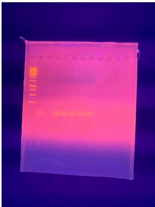
Figure 17: Electrophoresis gel results under UV light. The ladder was run on the farthest left well and the samples bands were run in the well to the right of it.
