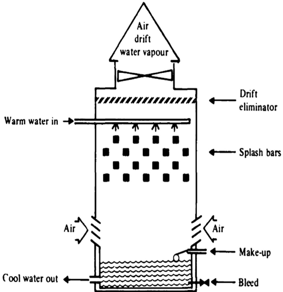
Figure 1: Schematic of cooling tower function (Kurtz et al., 1982).
