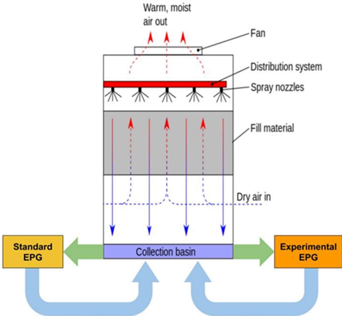
Figure 7: Split system treatment. Water in the collection basin is treated in one of the EPG units and returned to the collection basin (Edreher at English Wikipedia and Zerodamage, 2012). A modification was made to this image.
