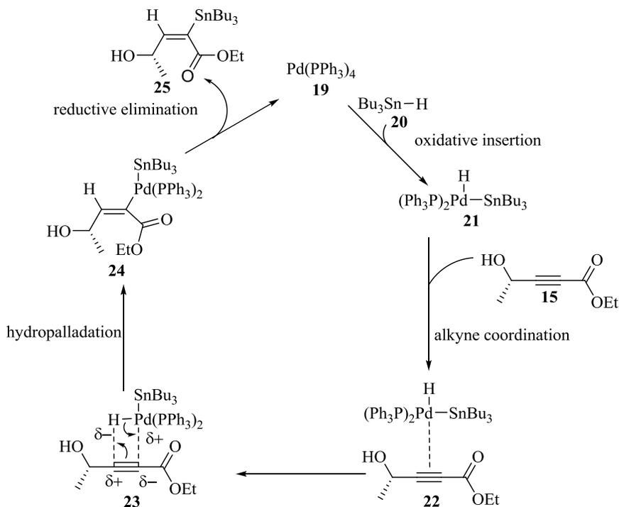
Scheme 4. Proposed mechanism of hydrostannylation to produce alkene **25** precursor to butenolide **7**
