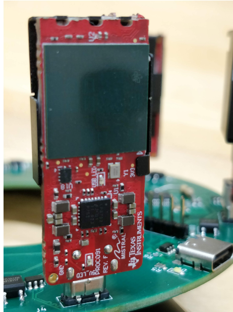
Figure 3.2: The Texas Instruments IWR6843AOP Rev F. with the debug portion broken off
