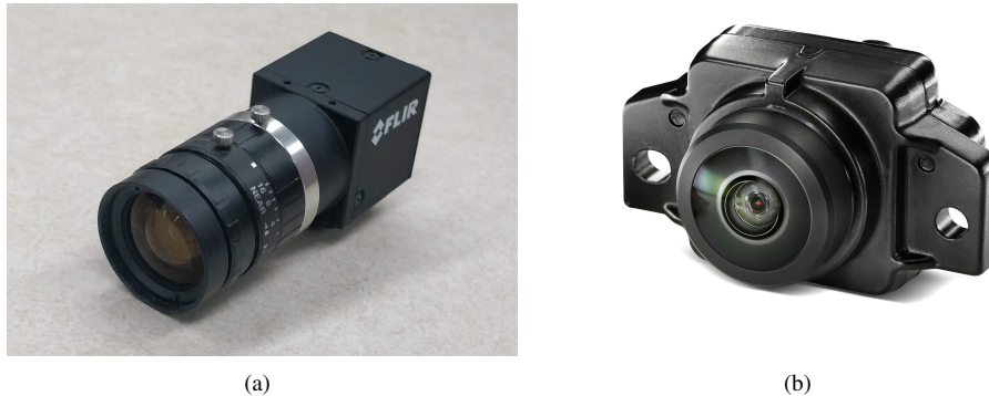
Figure 3.11: Cameras used for prototyping and testing: (a) Flir Flea 3 (b) D3 Engineering IMX390 rugged camera module
