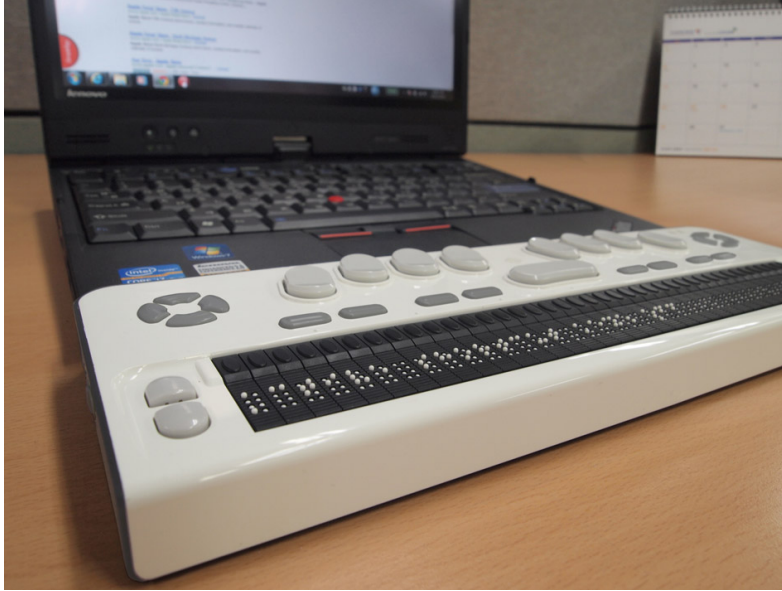
Figure 3.3: In this figure, we show an example of Braille Display device used by users with visual disabilities to access information on the computer display.
