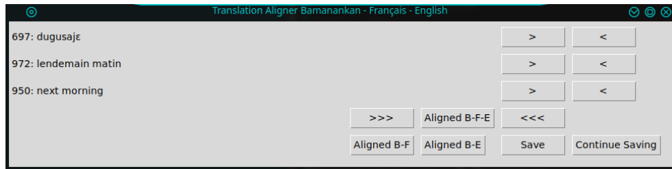
Figure 3.1: The custom aligner we developed to manually align the dictionary dataset. The controls are as follows: for each language, “>” goes to the next item and “<” goes to the previous item; for all languages, “>>>” goes to the next items and “<<<” goes to the previous items; “Aligned B-F-E” saves to memory the alignment of all 3 languages; “Aligned B-F” saves to memory the alignment of Bambara and French items; “Aligned B-E” saves to memory the alignment of Bambara and English items; “Save” saves to a new file; “Continue Saving” continues saving the file created.
