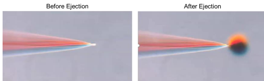
Figure 2-12: Before and after ejection of dye from the tip of a theta pipette into an aqueous environment.
