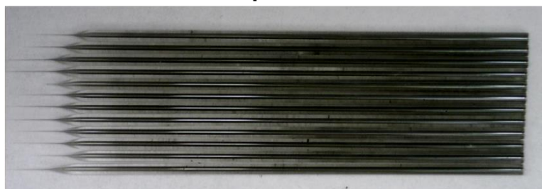
Figure 5-1: Effect of number of samples in CVD process on the amount of carbon deposited on template.
