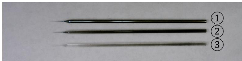
Figure 2-8: Effect of Ar:CH 4 ratio on carbon deposition.
