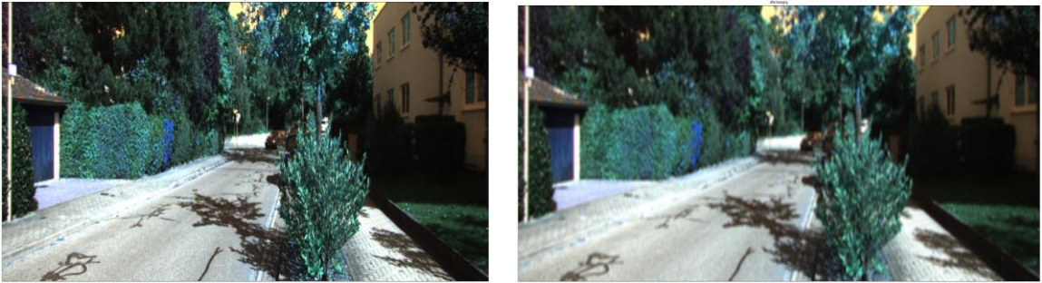
Figure 18: Effect of Average filer. Original Image (Left), Mean Filtered Image ( 5 \times 5 kernel)(Right)
