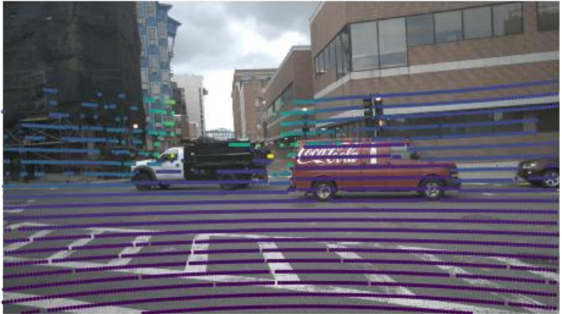
Figure 5: LiDAR point cloud overlaid on corresponding camera image.
