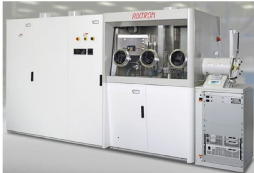
Figure 2.1: An Aixtron 3×2” CCS MOCVD reactor
