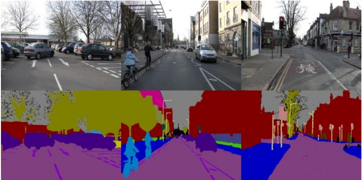
Figure 4.2: Sample images and pixel level labels from Camvid. Each image is taken from a car’s perspective.
