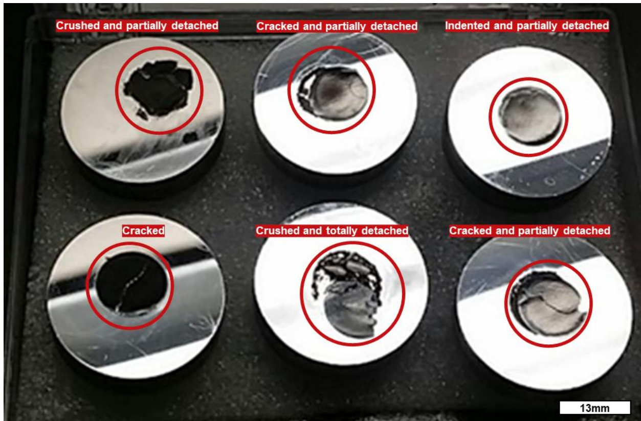
Figure 7: Failed polishing when mounted by tweezers.
