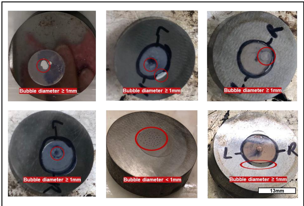
Figure 14: Air bubbles in different sizes and at different locations in the wax beneath the membrane.
