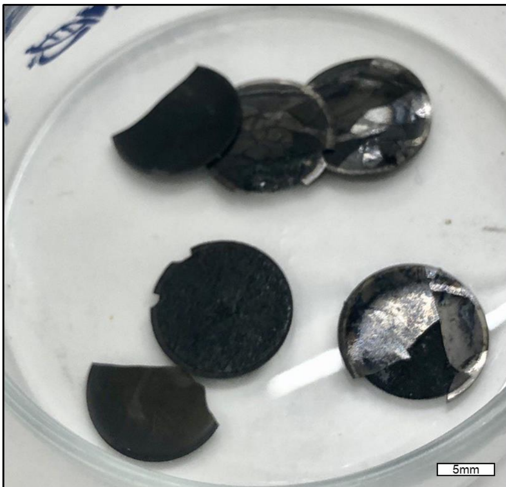
Figure 16: Membranes stick to carbon tape and break during detaching process.
