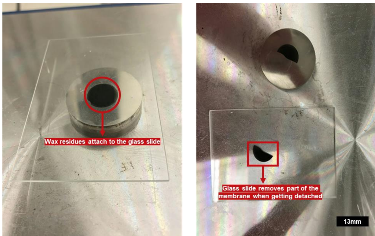
Figure 12: Glass slide experiment: applying the glass slide (left) and failure in removing it without damaging the membrane.
