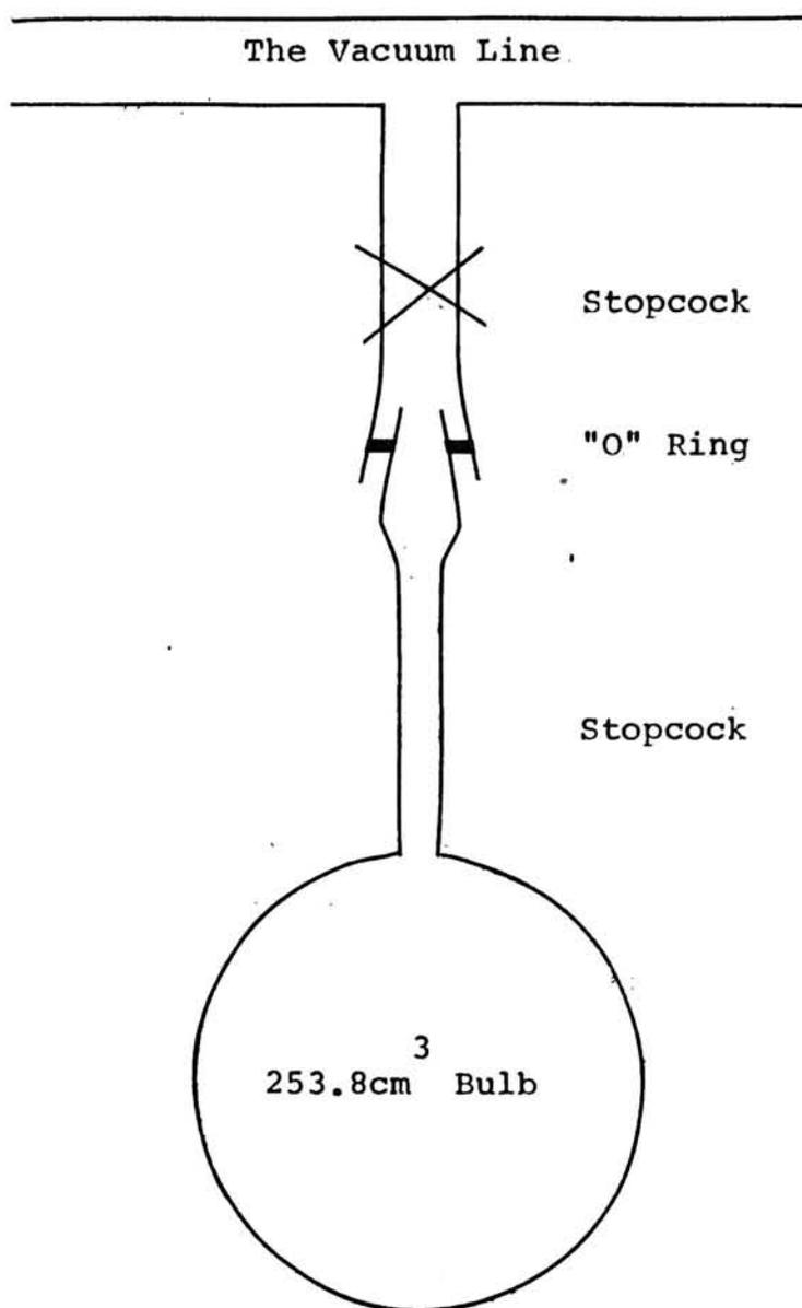
Figure 8. Molecular Weight Apparatus
