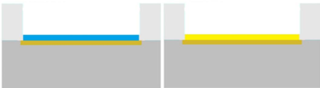
Figure 5.6 (e) Active area etch and deposition of Nickel (f) Formation of Nickel Silicide
