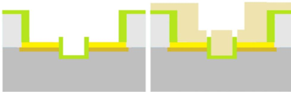
Figure 5.8 (i) Formation of Contact Cuts (j) Deposition and patterning of Aluminium metal
