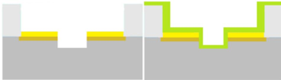
Figure 5.7 (g) Formation of V Shaped Recessed Channel (h) Deposition of PECVD Gate oxide
