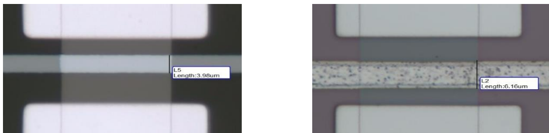
Figure 4.13: (a) SA-BG IGZO TFT with channel length L = 6 \mu\text{m} with effective channel length of L = 4 \mu\text{m} as defined by the subtractive wet etching using positive photoresist with 2 \mu\text{m} offset from the mask definition (i.e. \Delta L \sim 2 \mu\text{m} ) and (b) SA-TG IGZO TFT with channel length L = 6 \mu\text{m} as defined by the S/D lift-off metallurgy using negative photoresist (Futurrex NR9g-1500PY) with almost negligible offset from the mask definition (i.e. \Delta L \sim 0 ).
