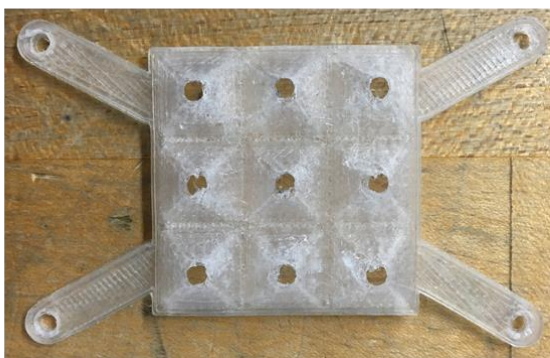
Figure 32. Volcano manifold, (a) No rewetting holes and (b) With rewetting holes.
