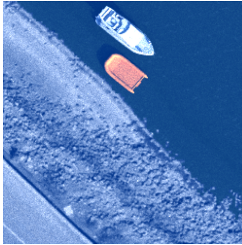
Figure 4.2: Example output from DIRSIG generated with high spatial resolution to show texture of materials within scene that was created using texture map (road and shore) and BRDF models (lifeboat and ship).
