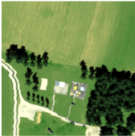
(c) A simulated image of the same scene generated using DIRSIG. Shown using three bands - R(650nm), G(550nm), and B(450nm).
