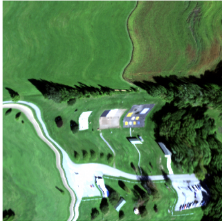
(a) A SHARE 2012 SpecTIR image of the scene used for the sub-pixel target detection experiment. Shown using three bands - R(650nm), G(550nm), and B(450nm).
